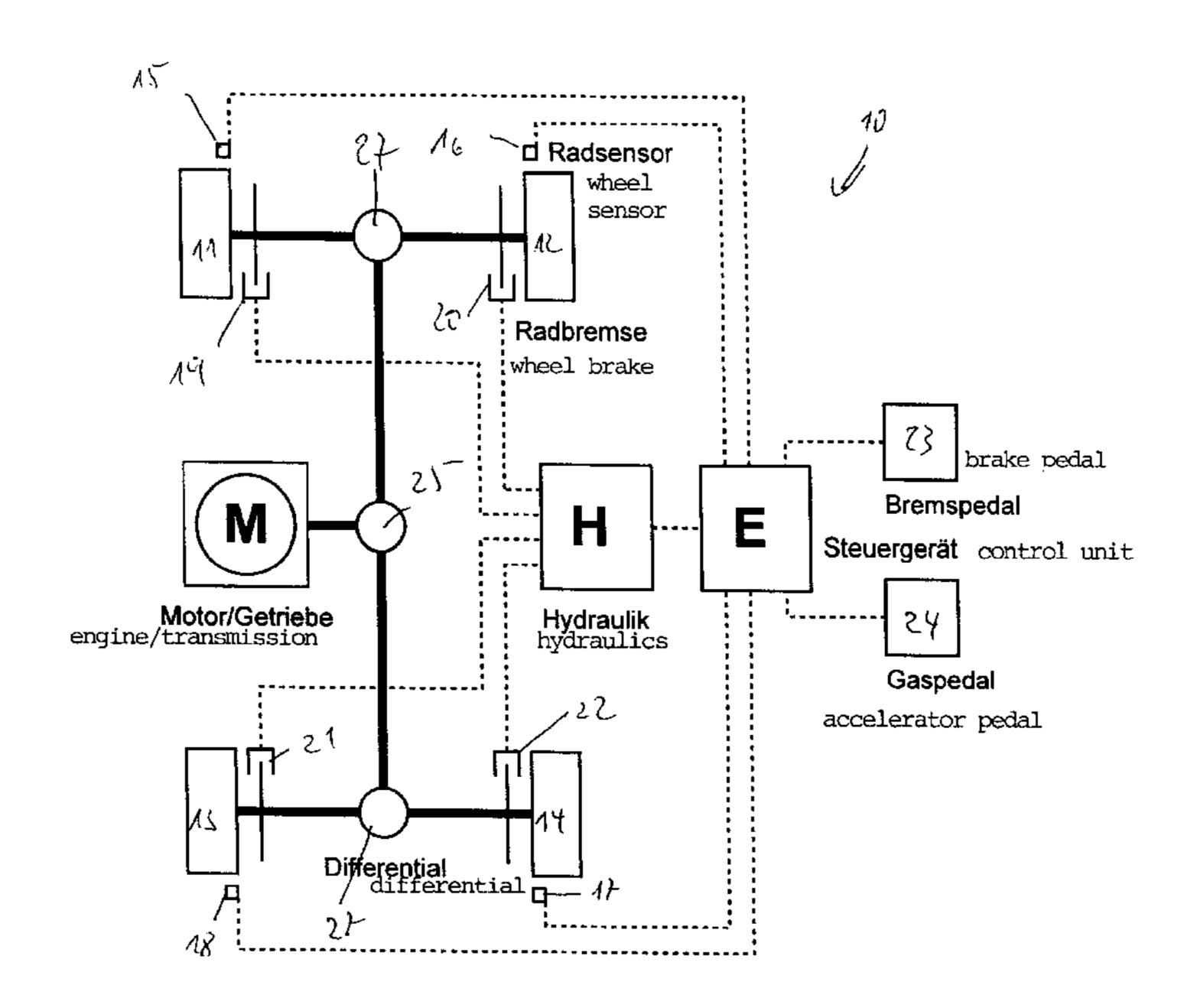
Fig. 1: Dragtorque Support DTS
