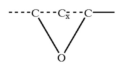
wherein x is zero or a whole number, typically from 1 to 4, such that the epoxide functionality of the epoxy resin is equal to or greater than 2.0, typically from 2.3 to 3.5. Although an epoxy resin may contain some monomeric bisphenol A and bisphenol F, the term "epoxy resin" should not be construed as pure monomeric bisphenol A and bisphenol F, which have an epoxide functionality of 2.0.
