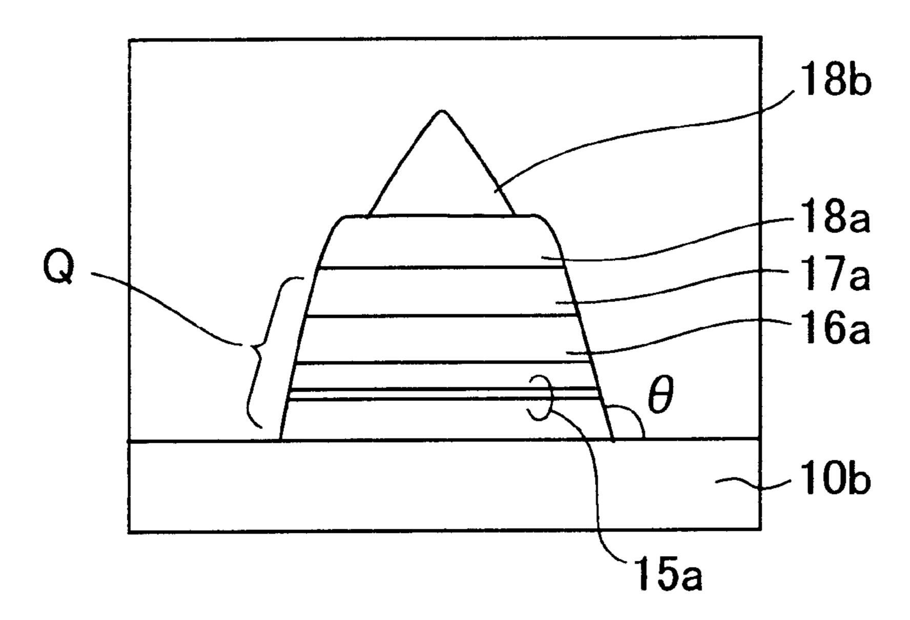
WAFER STAGE TEMPERATURE: 300°C TAPER ANGLE  $\theta$  OF A SIDE FACE: 76°
