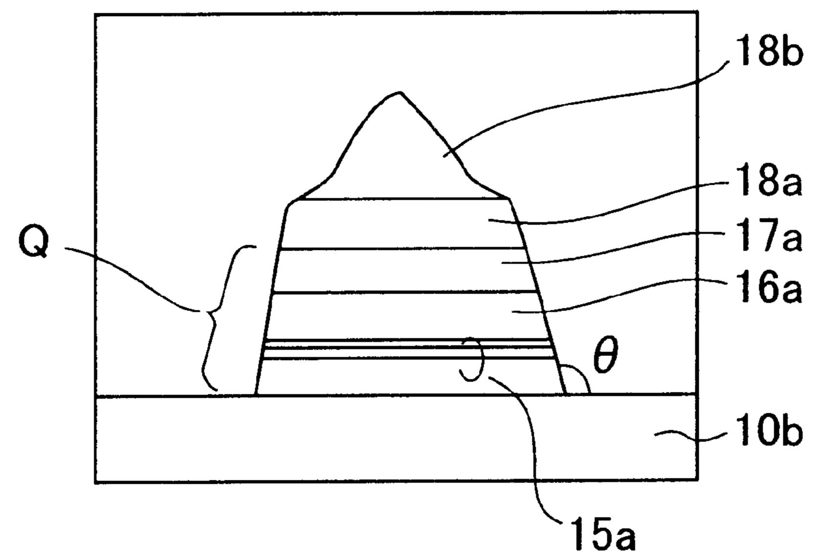
WAFER STAGE TEMPERATURE: 400°C TAPER ANGLE  $\theta$  OF A SIDE FACE: 79°
