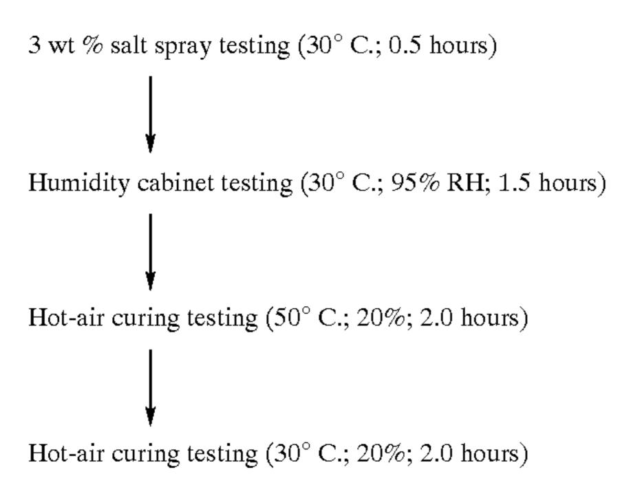
The evaluation was performed for the rust-developed area ratio in 5-mm areas on two sides of the cut slit. The conditions (color tones) of developed rust depended on the Al concentration of the plating film. White rust was caused in zinc-plated steel sheets and Zn/Al-base-plated steel sheets 25 having Al concentrations of at most 25 wt %. Rust ranging in color from gray to black was caused on Zn/Al-base-plated steel sheets having Al concentrations ranged from 25 to 75 wt %.
