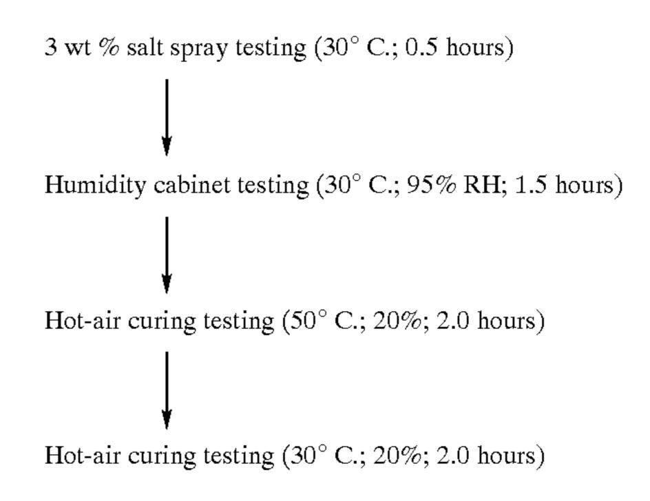
The evaluation was performed for the rust-developed area ratio in 5-mm areas on two sides of the cut slit. The conditions (color tones) of developed rust depended on the Al concentration of the plating film. White rust was caused in zinc-plated steel sheets and Zn/Al-base-plated steel sheets having Al concentrations of at most 25 wt %. Rust ranging in color from gray to black was caused on Zn/Al-base-plated steel sheets having Al concentrations ranged from 25 to 75 wt %.
