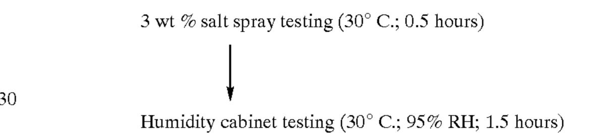
Using the same criteria as those in Example 1, evaluation was performed for the rust-developed area ratio in 5-mm areas on two sides of the cut slit. The conditions (color tones) of developed rust were the same as in the case of the evaluation of the processed-portion corrosion resistance in Example 1.
