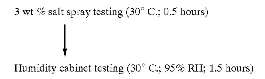
Using the same criteria as those in Example 1, evaluation was performed for the rust-developed area ratio in 5-mm areas on two sides of the cut slit. The conditions (color tones) of developed rust were the same as in the case of the evaluation of the processed-portion corrosion resistance in Example 1.
