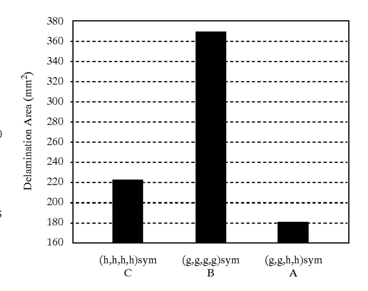
This shows that the structure according to the invention exhibits the smallest delamination area.
