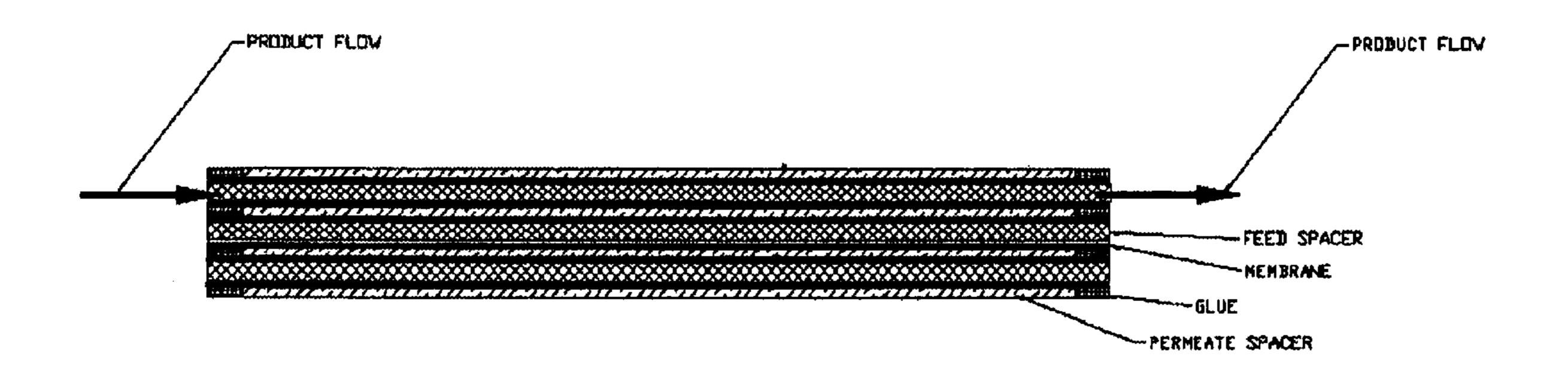
CUT-AWAY VIEW OF THREE CHANNELS OF A STANDARD SPIRAL WOUND MODULE
