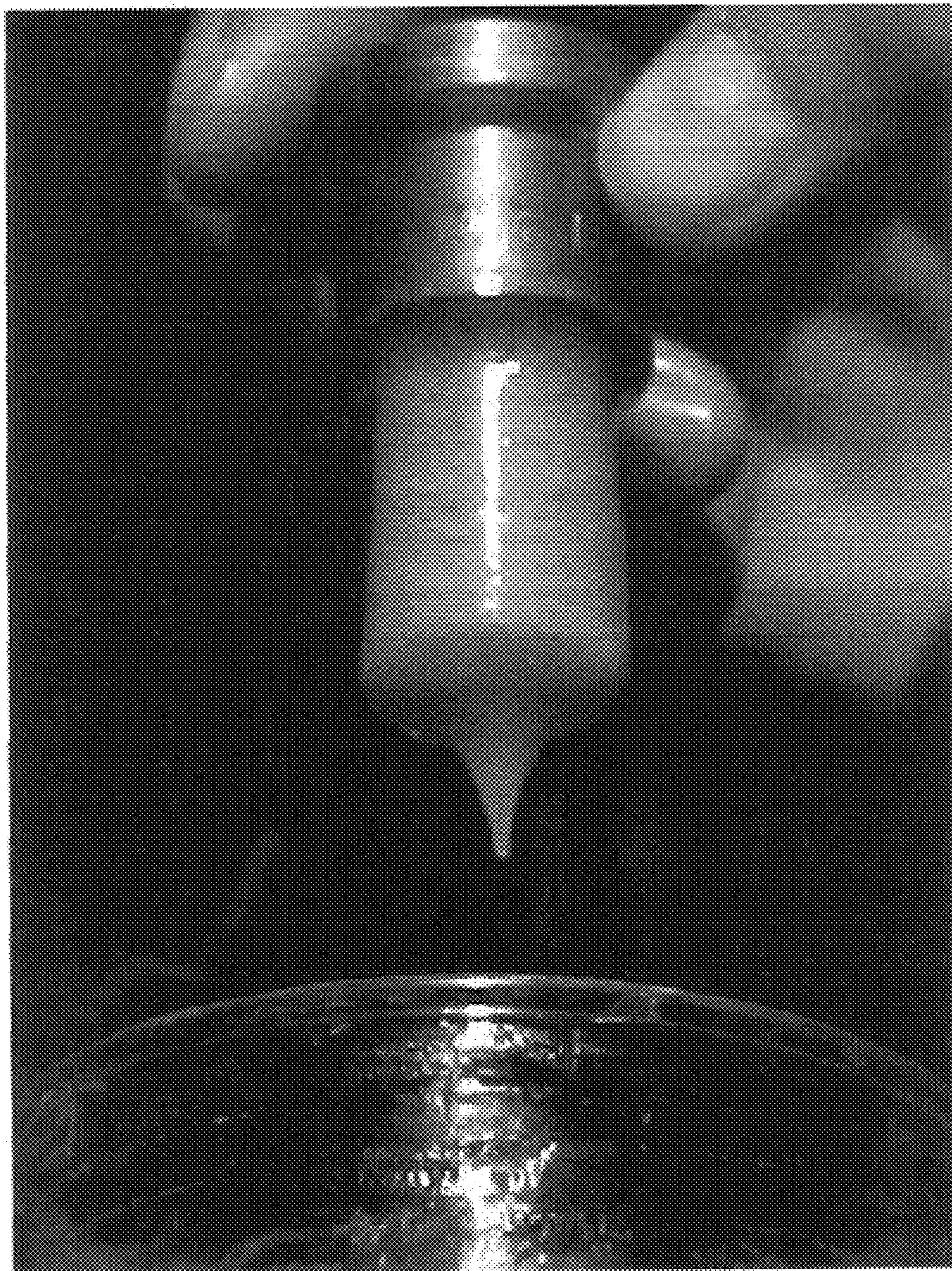
Figure 7- Modified Lubricant Showing Clingage to the Surface
