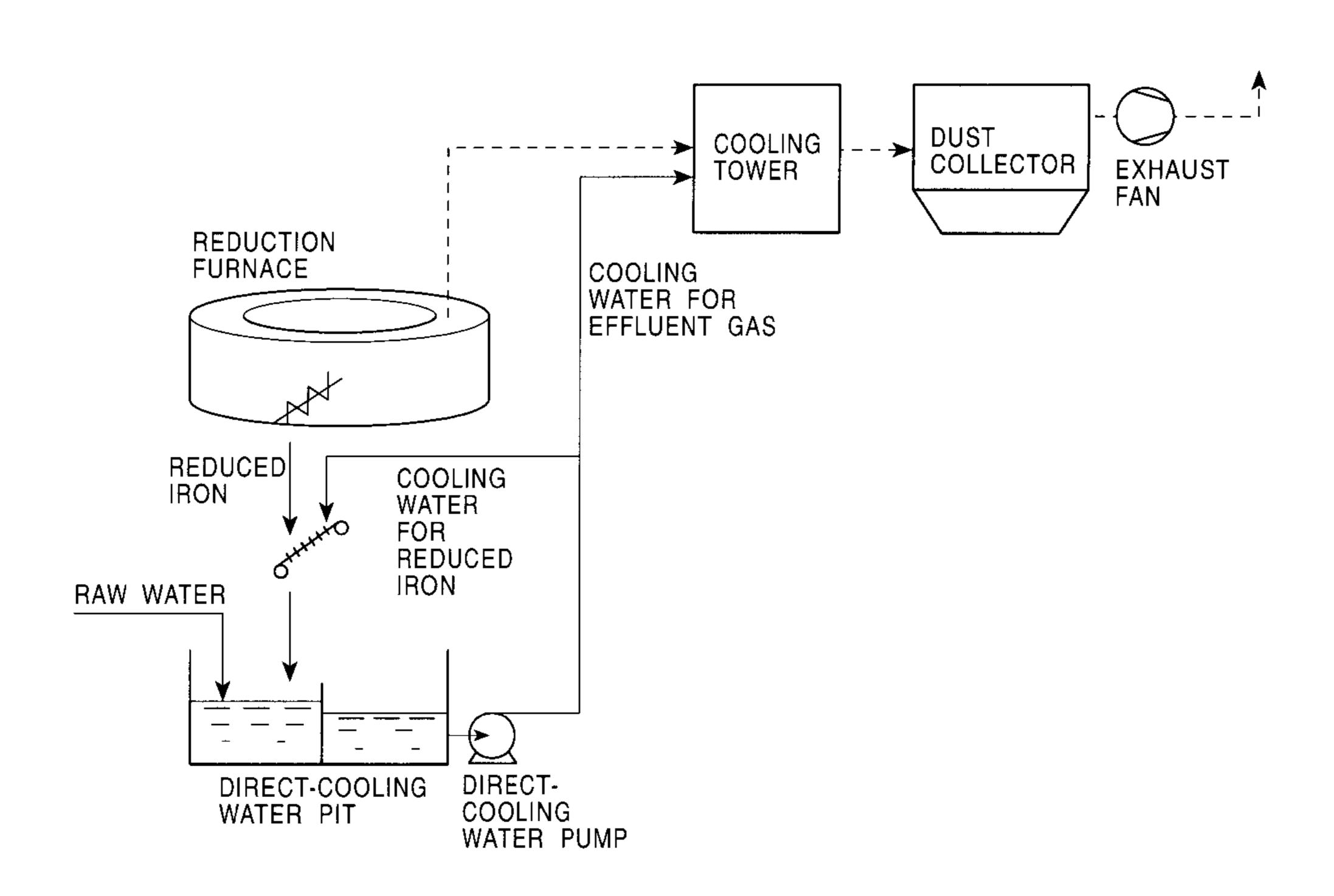
EXH COOLING WATER FOR EFFLUENT GAS DIRECT-COOLING WATER PIT REDUCTION FURNACE WATER
