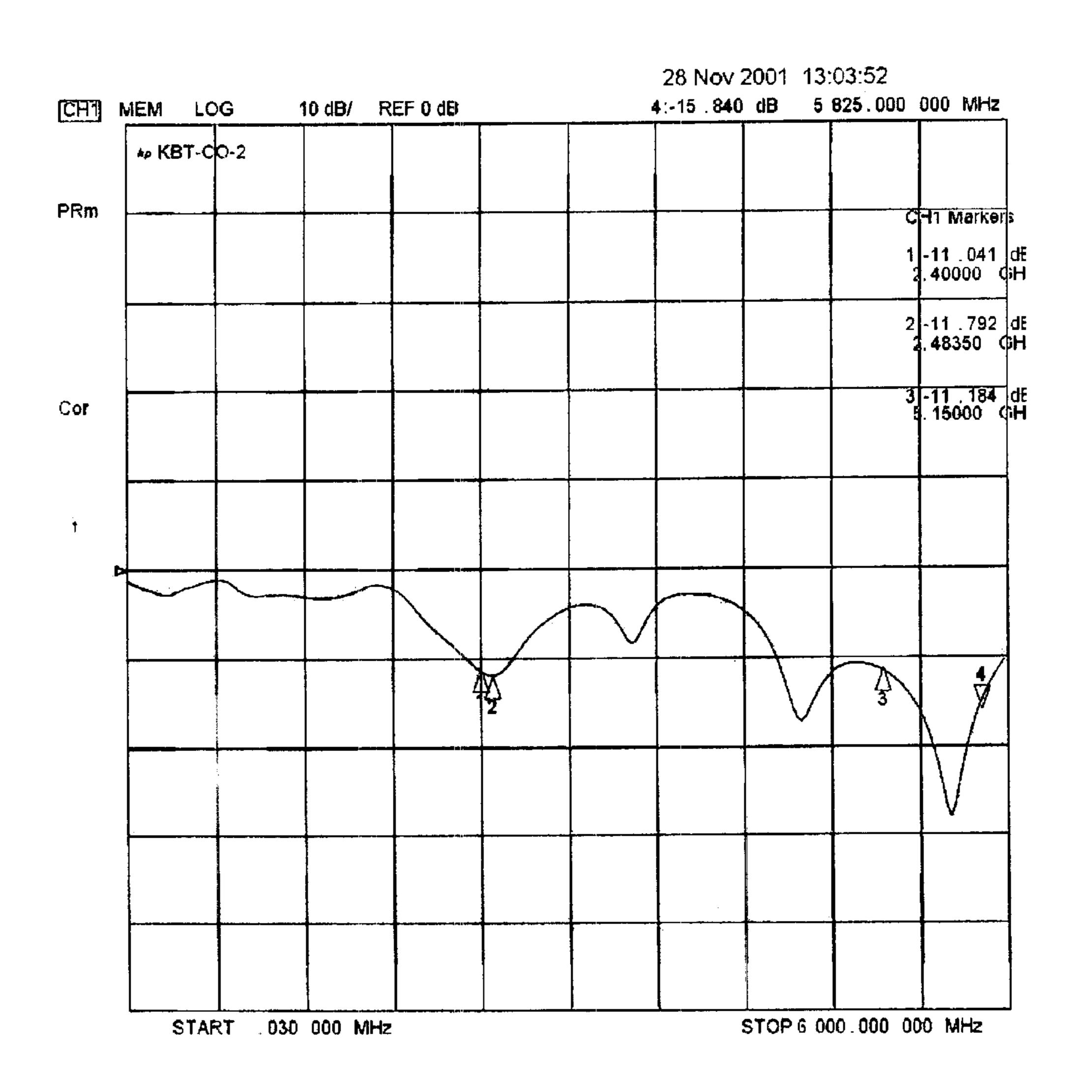
Marker 1: 2.40000 GHz Marker 2: 2.48350 GHz Marker 3: 5.15000 GHz Marker 4: 5.82500 GHz
