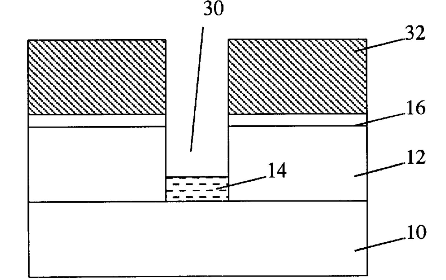
Etching organic low-k dielectric using silyated photoresist as an etch mask and oxidation of silyated photoresist
