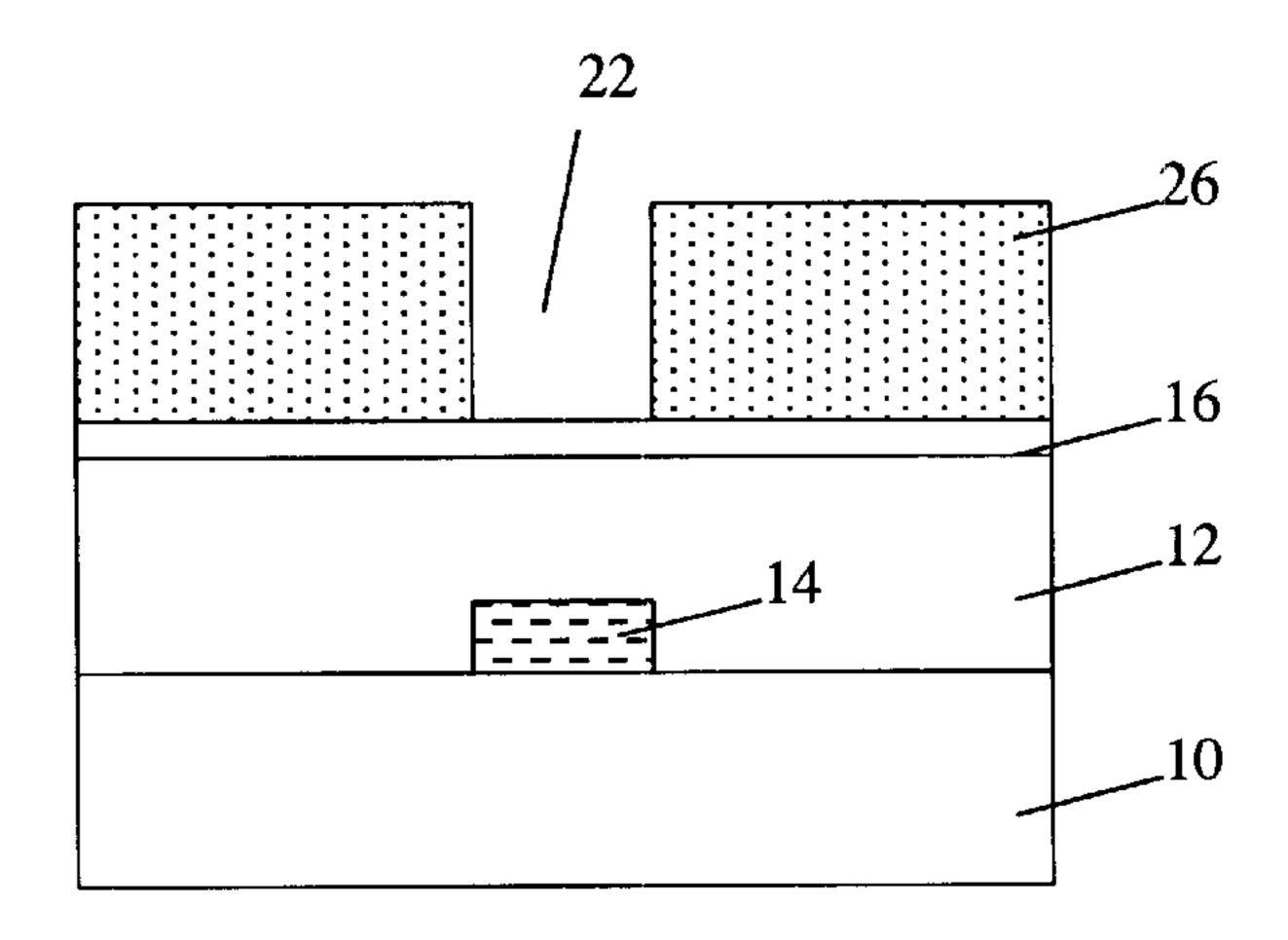
Figure 5 Etching hardmask using silyated photoresist as an etch mask
