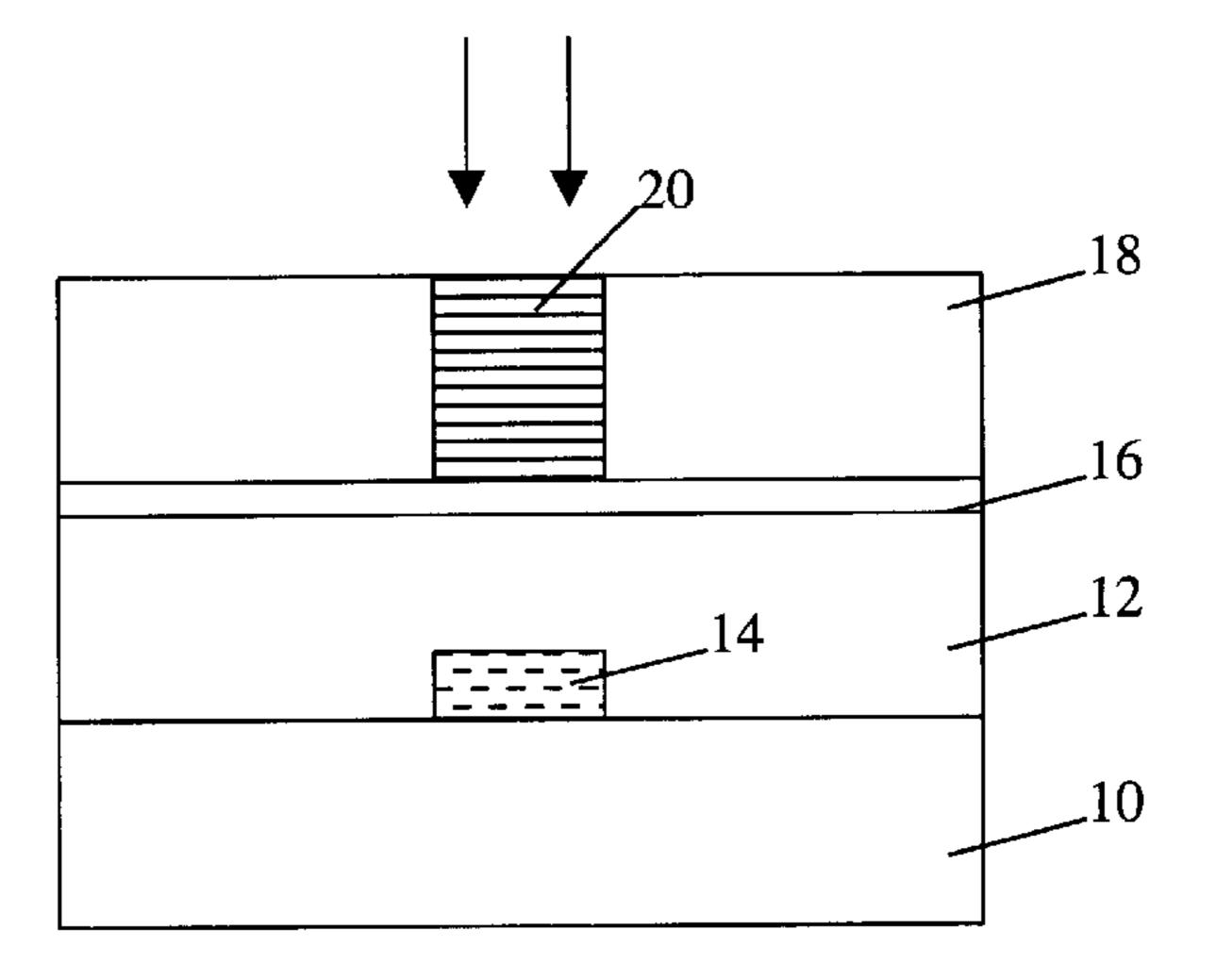
Figure 3 Photoresist development
