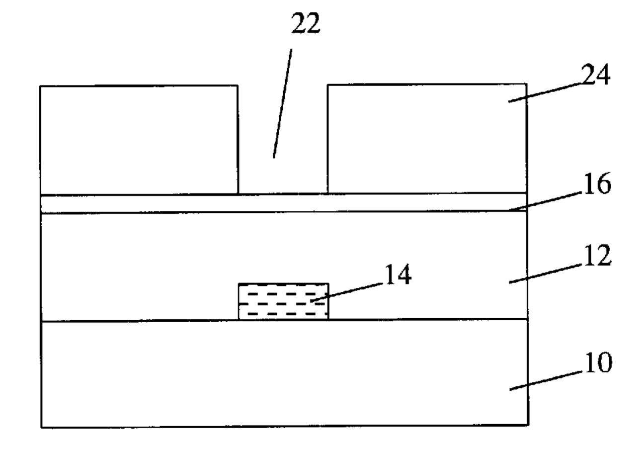
Figure 4 Silyation of photoresist
