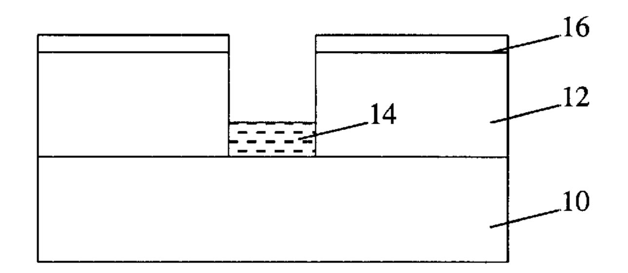
Figure 8 Filling void with metal to form contact
