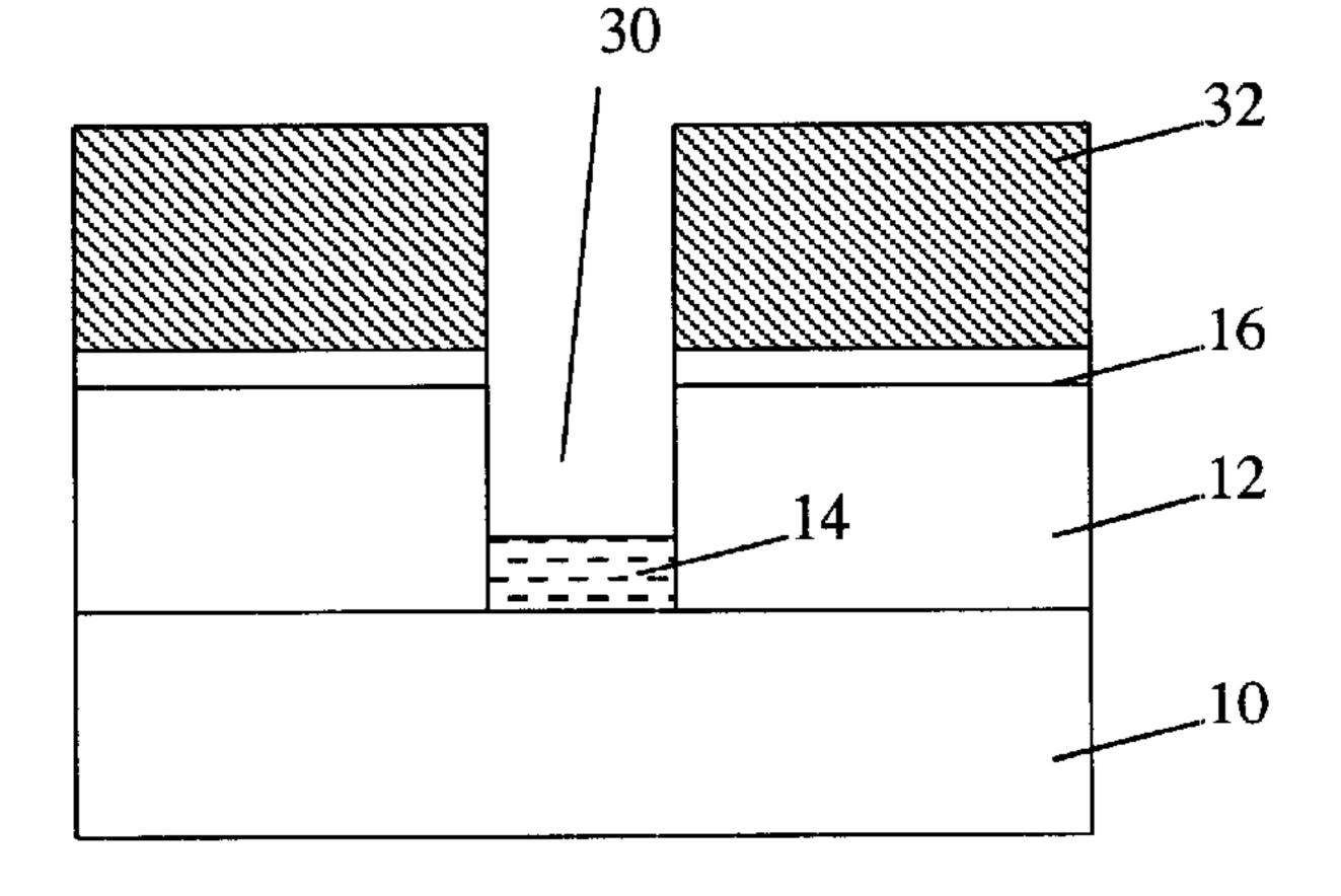
Figure 7 Stripping silicon oxide etch mask
