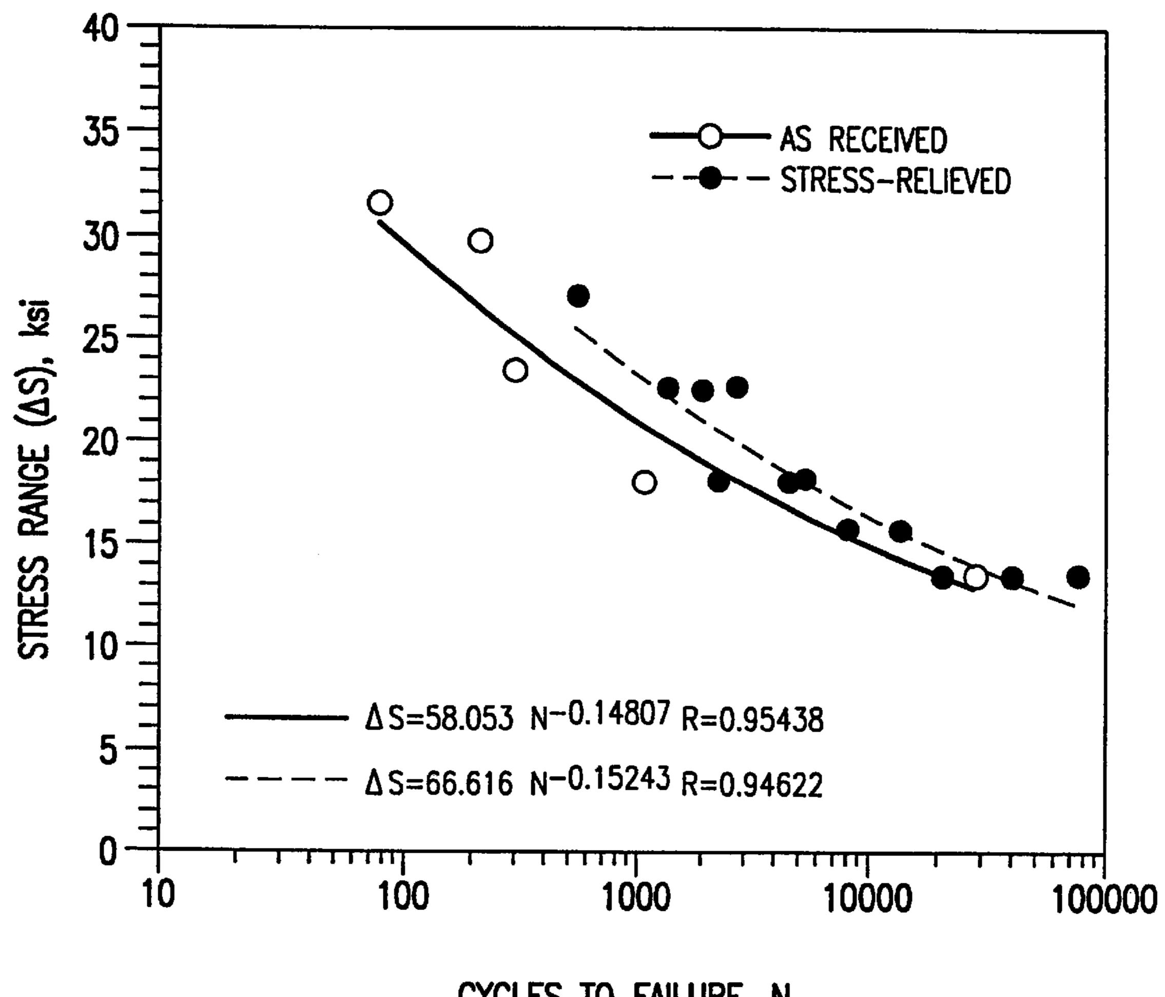
CYCLES TO FAILURE, N
