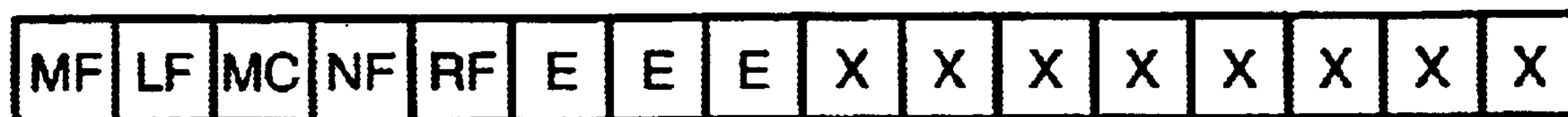
FIG. 7 - Sixteen Bit Control Field Format
