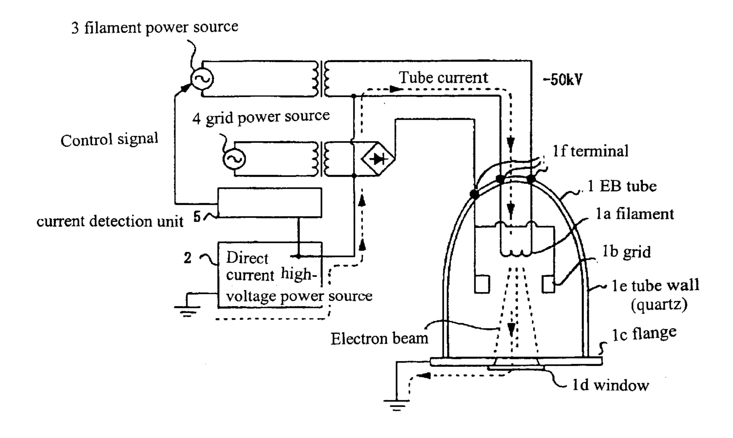
A diagram explaining the disposition of the window of an EB tube.
