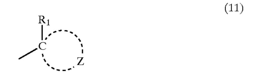
where R<sub>1</sub> is an alkyl group of a straight chain or branched chain containing one to four carbon atoms, or a replacement group of the alkyl group, and Z is an atom group constituting an alicyclic hydrocarbon group together with the carbon atom bonded to  $R_1$ .
