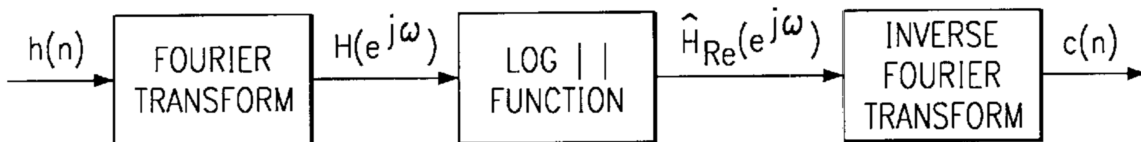
FIG. 6a \text{Log}|H(e^{j\omega})| = \hat{H}_{Re}(e^{j\omega})
