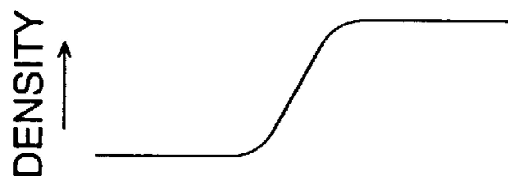
(b) CROSS SECTION OF BLURRED EDGE
