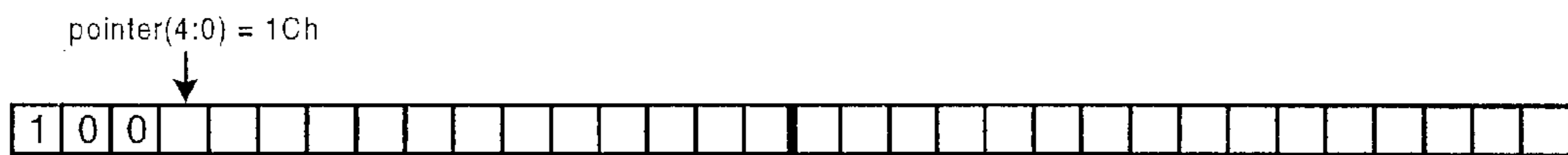
Fig. 2 example bit-packing buffer after packing code '100'
