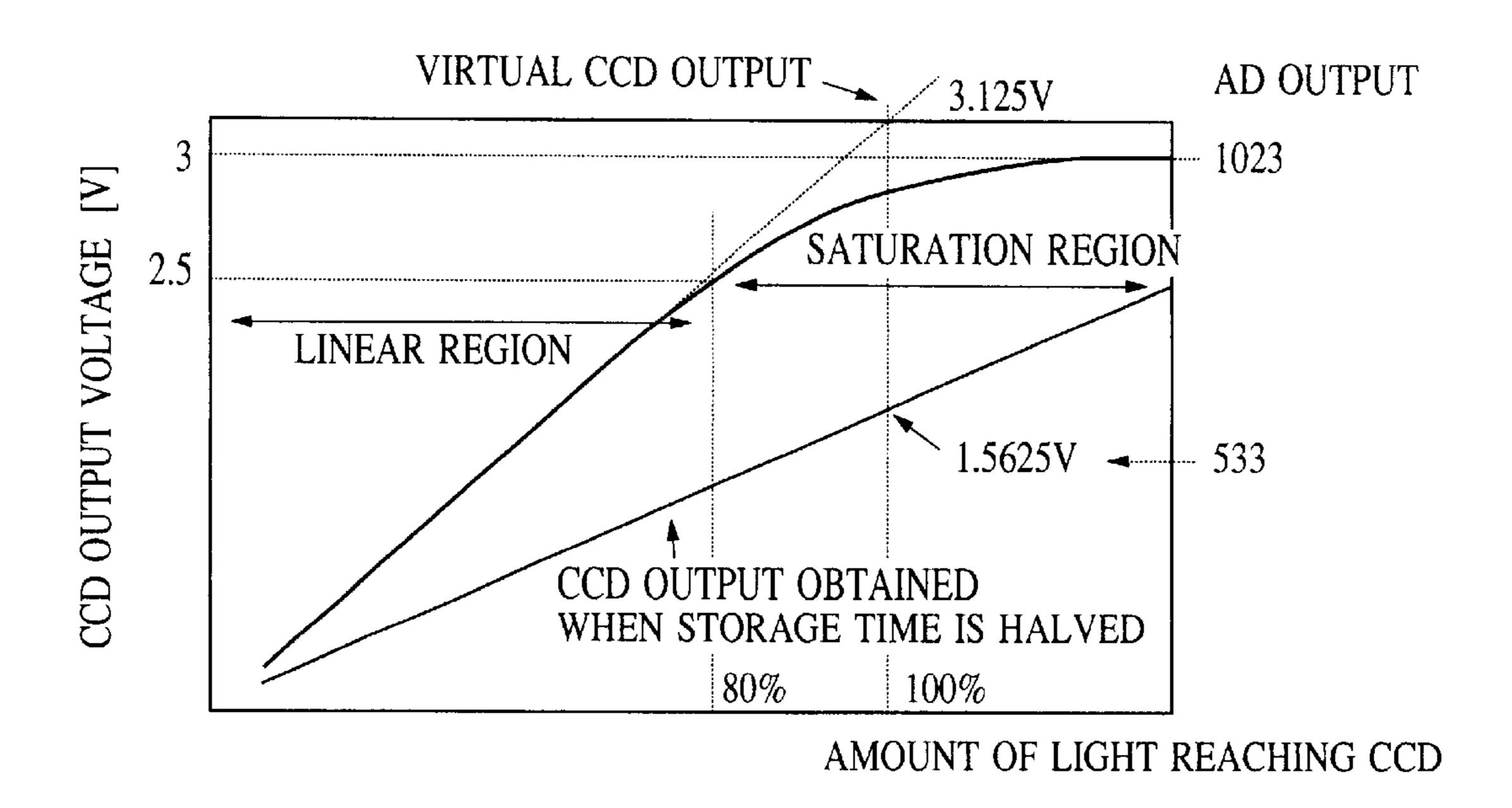
RELATIONSHIP BETWEEN CCD PHOTOELECTRIC CONVERSION RANGE AND AD CONVERTER OUTPUT
