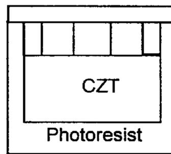
Step4 Gold is deposited on substrate
