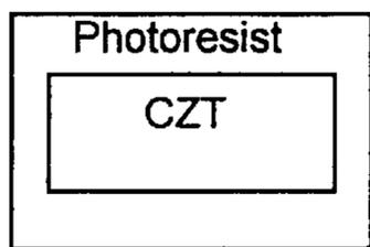
Step1 Spin Photoresist on CZT
