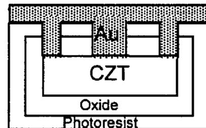
Step6 Gold is deposited on substrate
