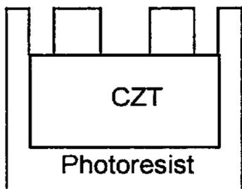
Step3 Photoresist is developed
