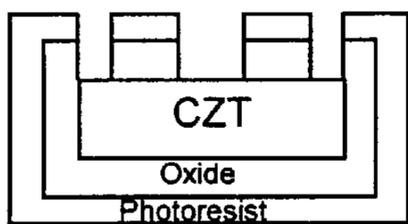
Step5 Oxide is etched through pattern photoresist
