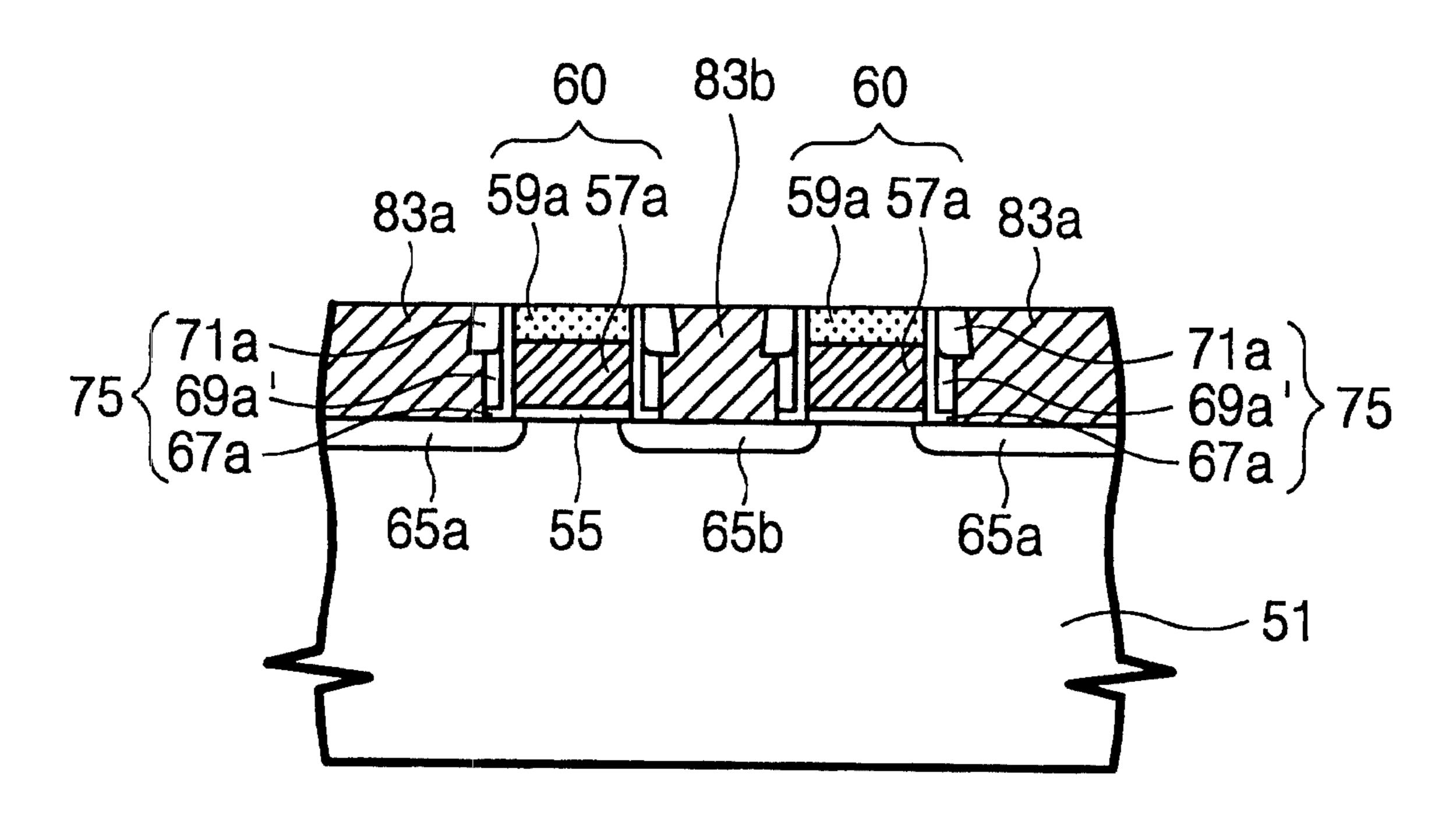
METHODS FOR FORMING INTEGRATED CIRCUIT DEVICES THROUGH SELECTIVE ETCHING OF AN INSULATION LAYER TO INCREASE THE SELF-ALIGNED CONTACT AREA ADJACENT A SEMICONDUCTOR REGION AND INTEGRATED CIRCUIT DEVICES FORMED THEREBY
