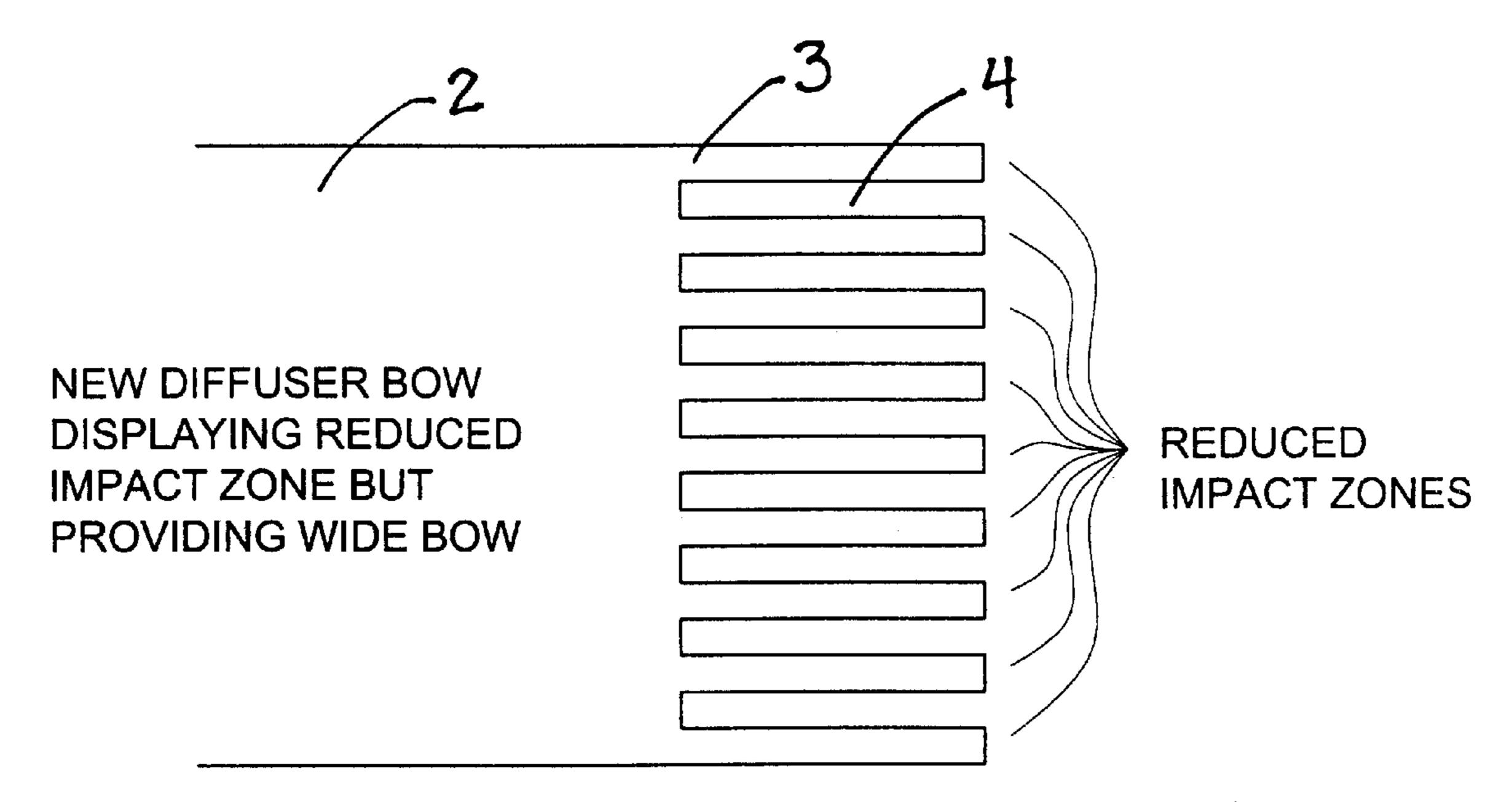
DIFFUSER PROVIDES AIR CHANNELS TO LESSEN IMPACT THROUGH COMPRESSION OF AIR AND WATER MIXTURE AND REDUCTION OF SUCTION ON HULL
