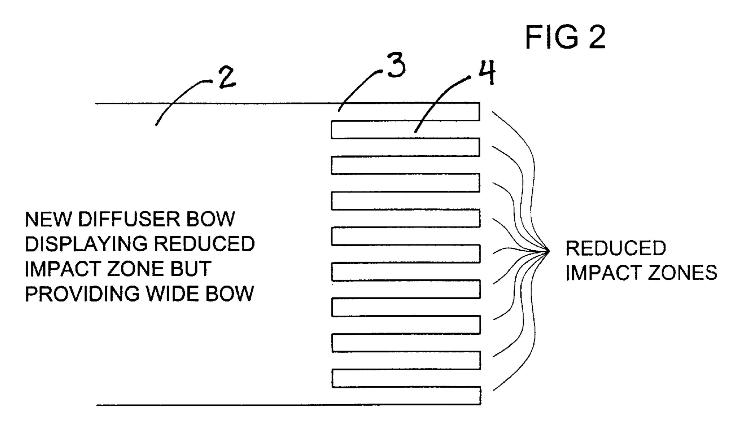
DIFFUSER PROVIDES AIR CHANNELS TO LESSEN IMPACT THROUGH COMPRESSION OF AIR AND WATER MIXTURE AND REDUCTION OF SUCTION ON HULL
