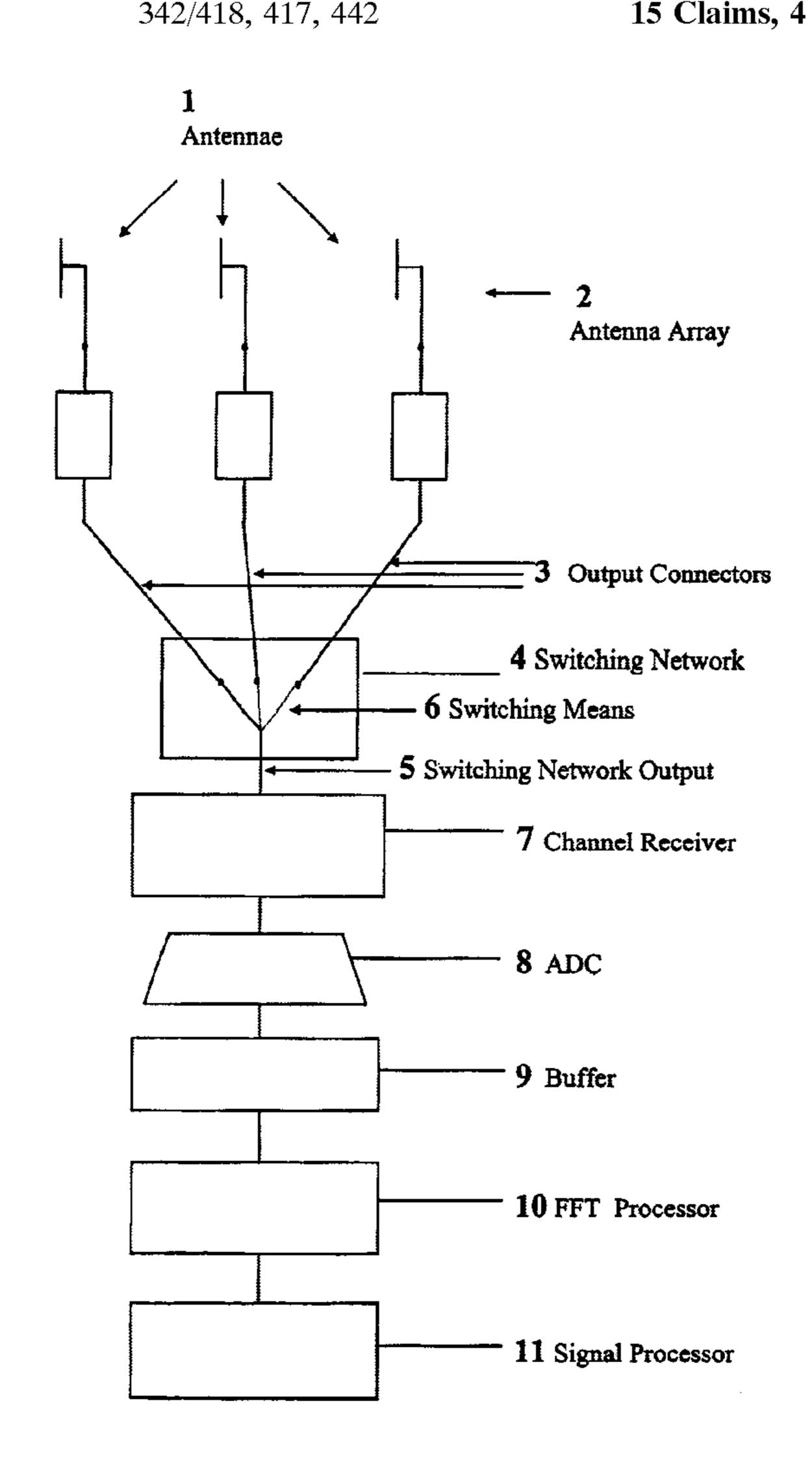
Figure 1 Antennae Antenna Array Output Connectors 4 Switching Network 6 Switching Means 5 Switching Network Output 7 Channel Receiver 8 ADC 9 Buffer 10 FFT Processor - 11 Signal Processor
