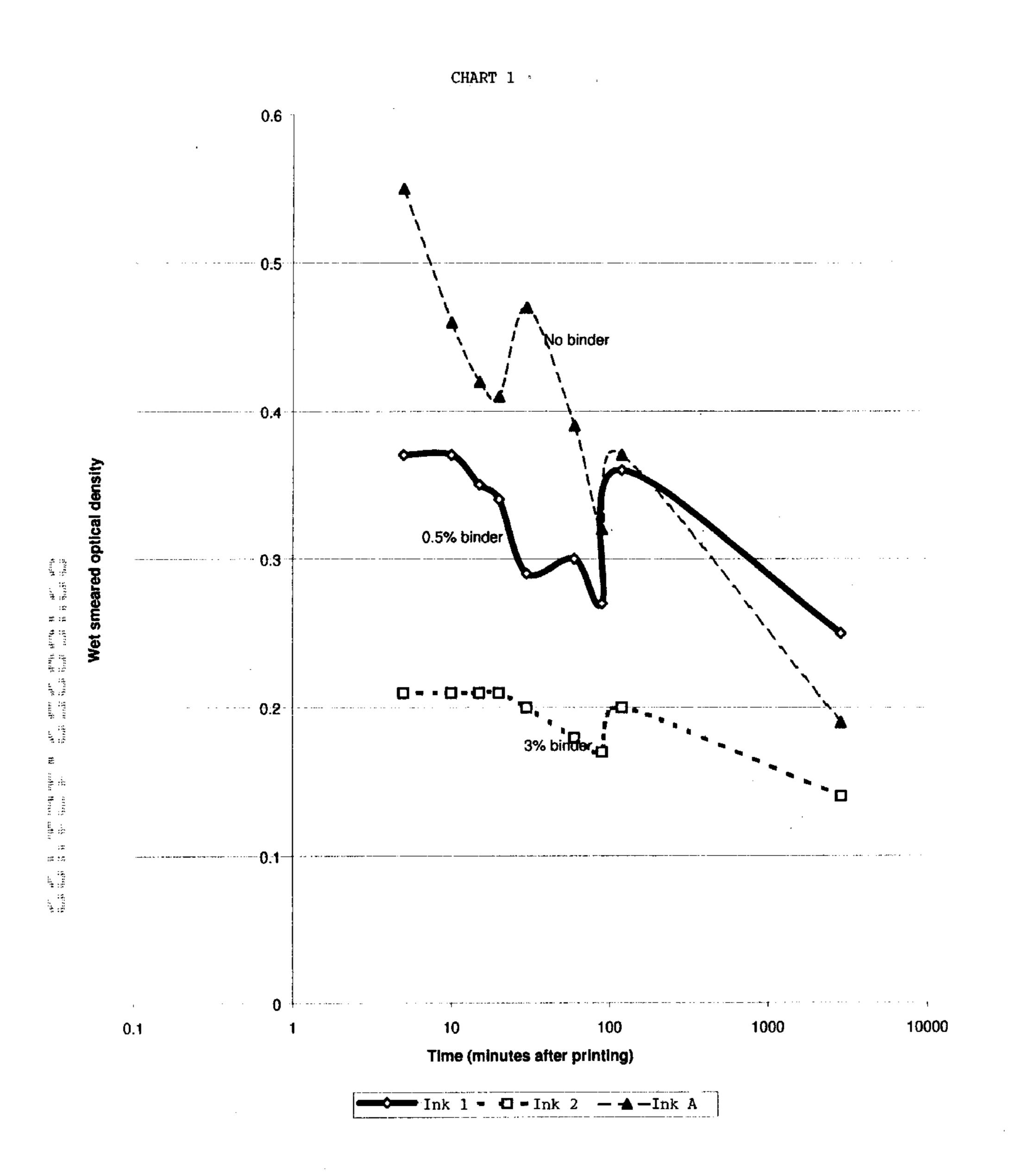
The resistance of Ink Compositions 1, 2, 3, A and B to highlighter smear was determined by using a commercially available densitometer to measure the optical density of the
