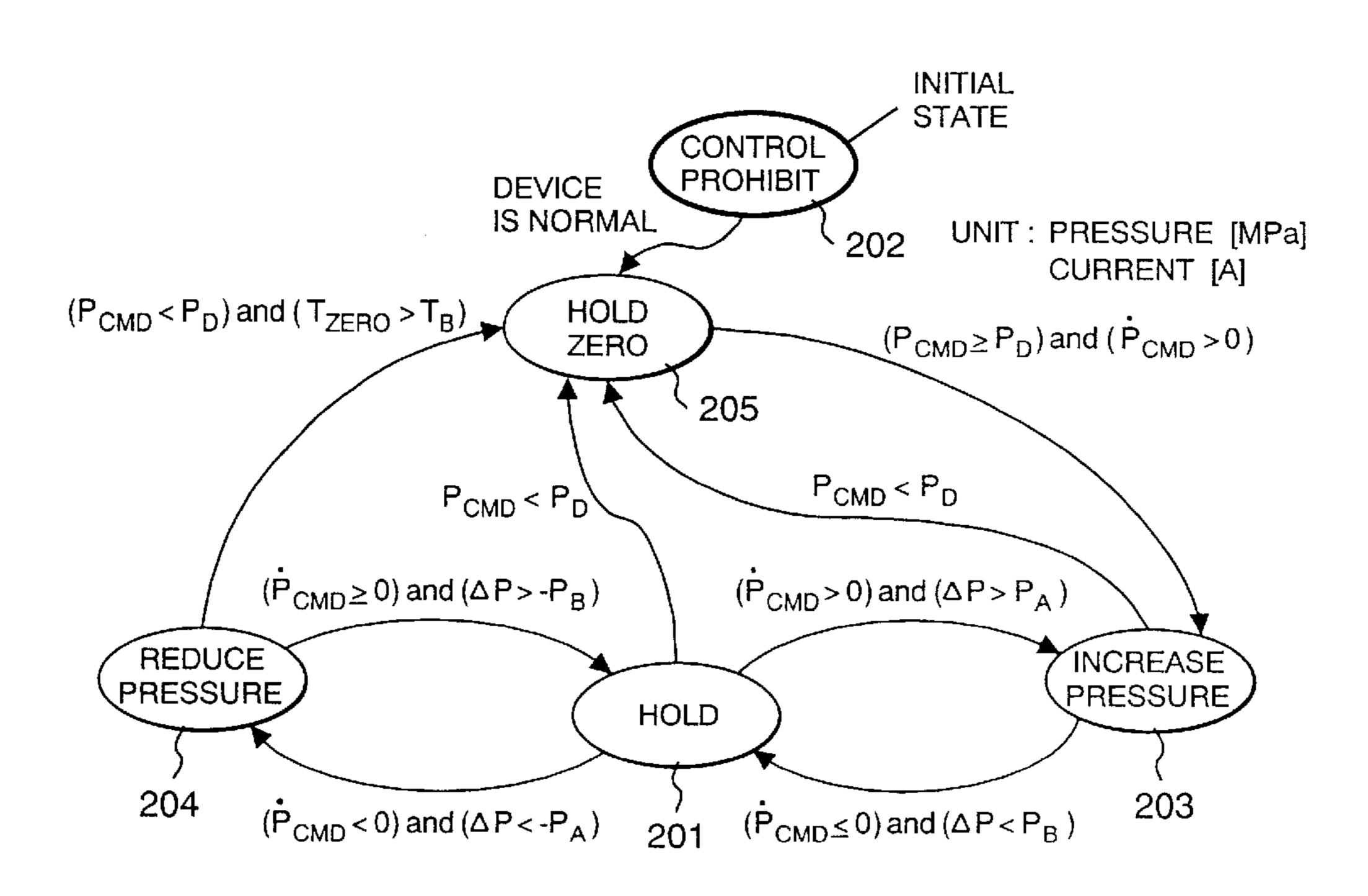
WHEN "DEVICE IS FAULTY" IS DECIDED IN ALL STATES, A TRANSITION IS MADE TO "CONTROL PROHIBIT"
