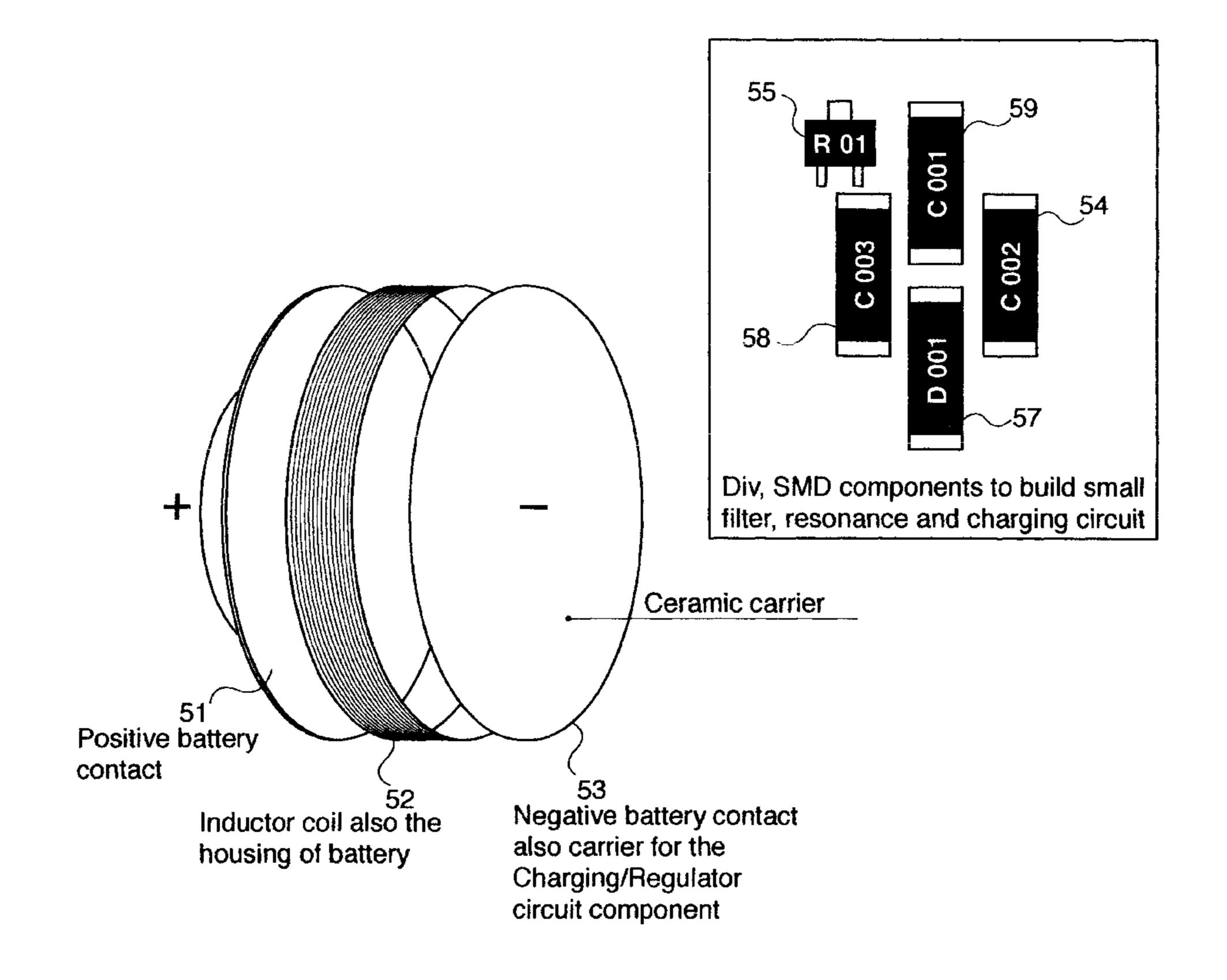
small circuit components to build charging 9 C 005 and C 001 100 a resonance o C 003 COI Div, SMD inductor filter, Mounted inside gy inducting component Ceramic carrier
