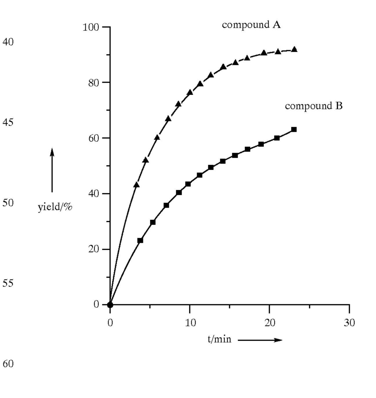
ROMP of cyclooctene. NMR kinetics of a ruthenium-dicarbene complex compared to a ruthenium-carbene-phosphine complex. (T=25° C.; 2.50 µmol of catalyst in 0.50 ml of CD<sub>2</sub>Cl<sub>2</sub>; [cyclooctene]/[catalyst]=250:1.
