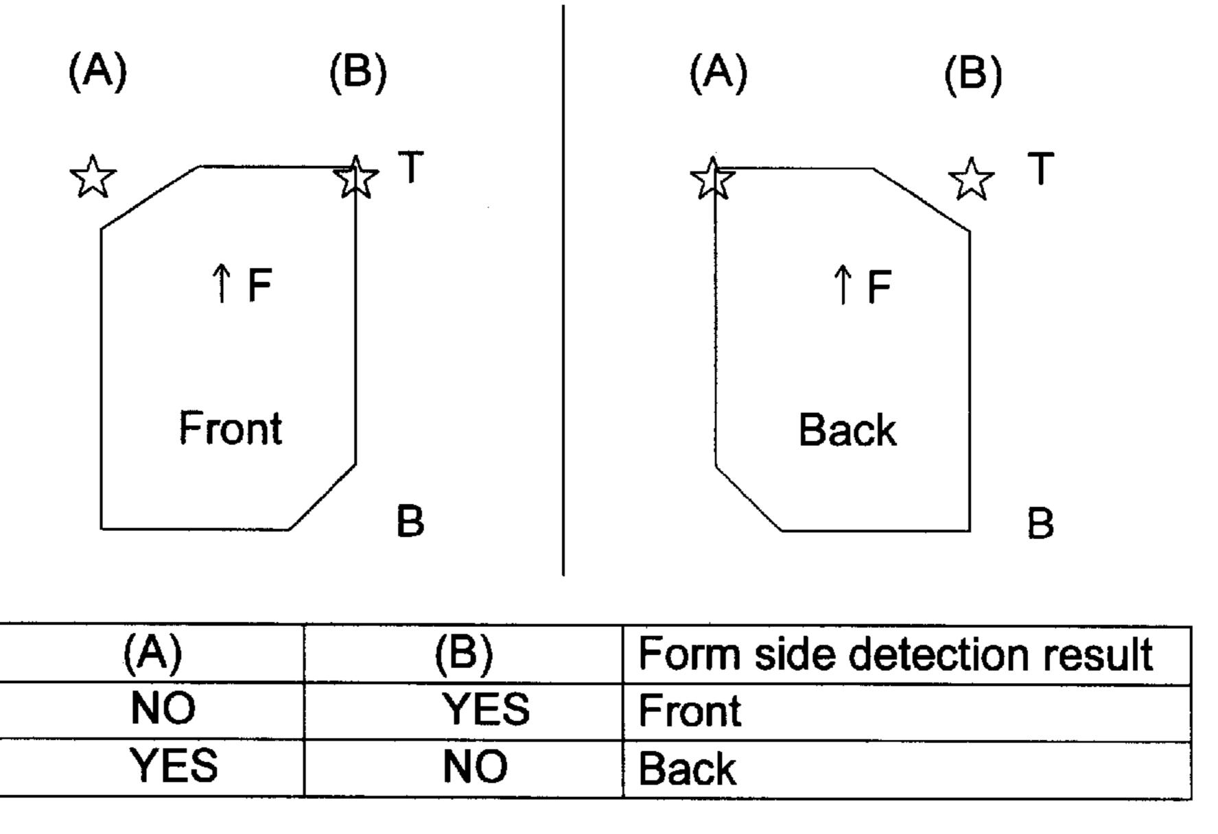
[A,B:Detector/(star):Detector position/YES:Form detected/NO:Form not detected]
