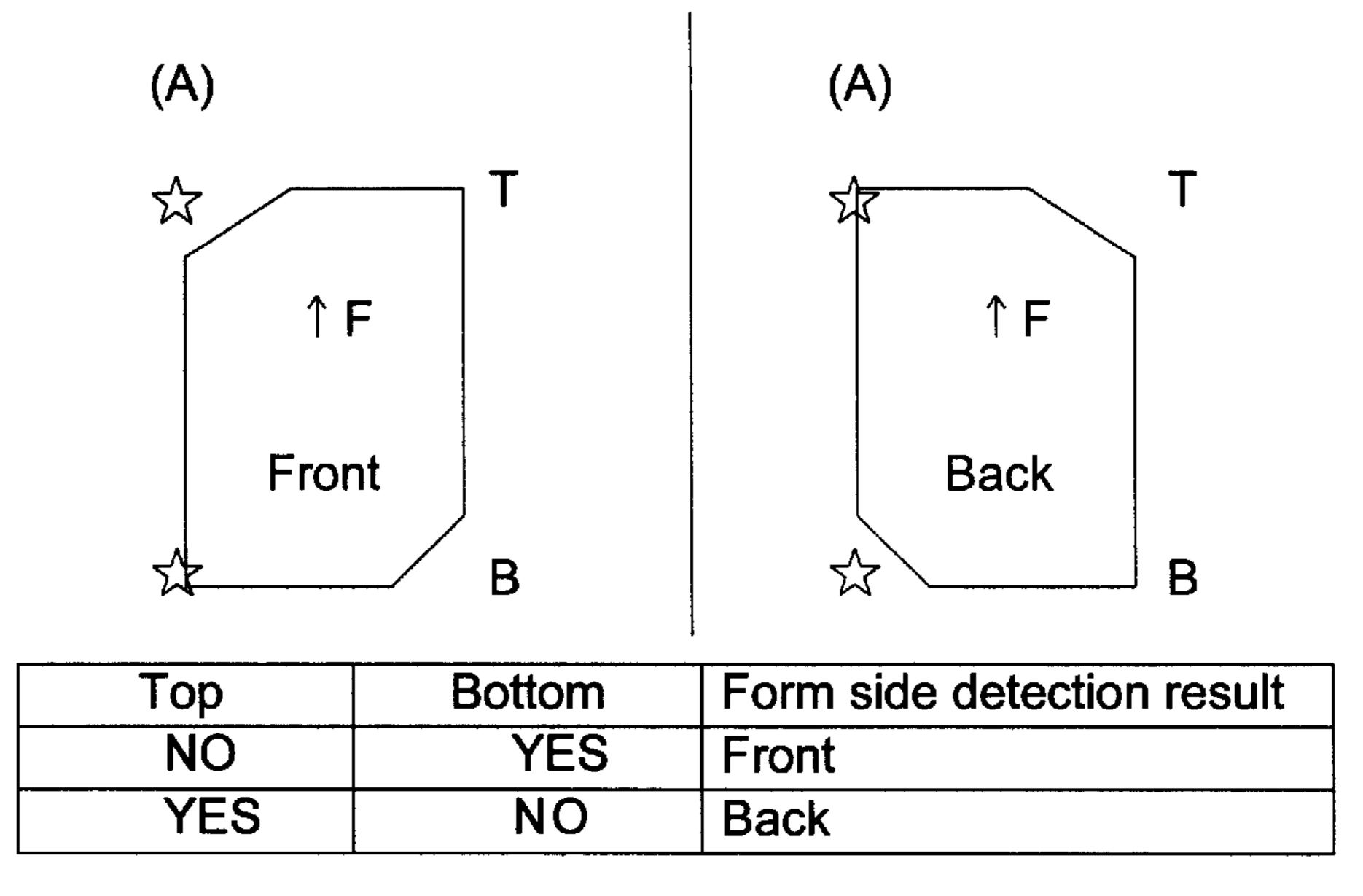
[A :Detector/(star):Detector position/YES:Form detected/NO:Form not detected]
