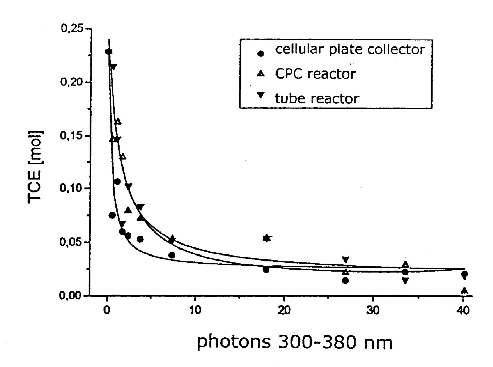
Degradation of TCE in water (500 mg/l), catalyst TiO<sub>2</sub> (200 mg/l)
