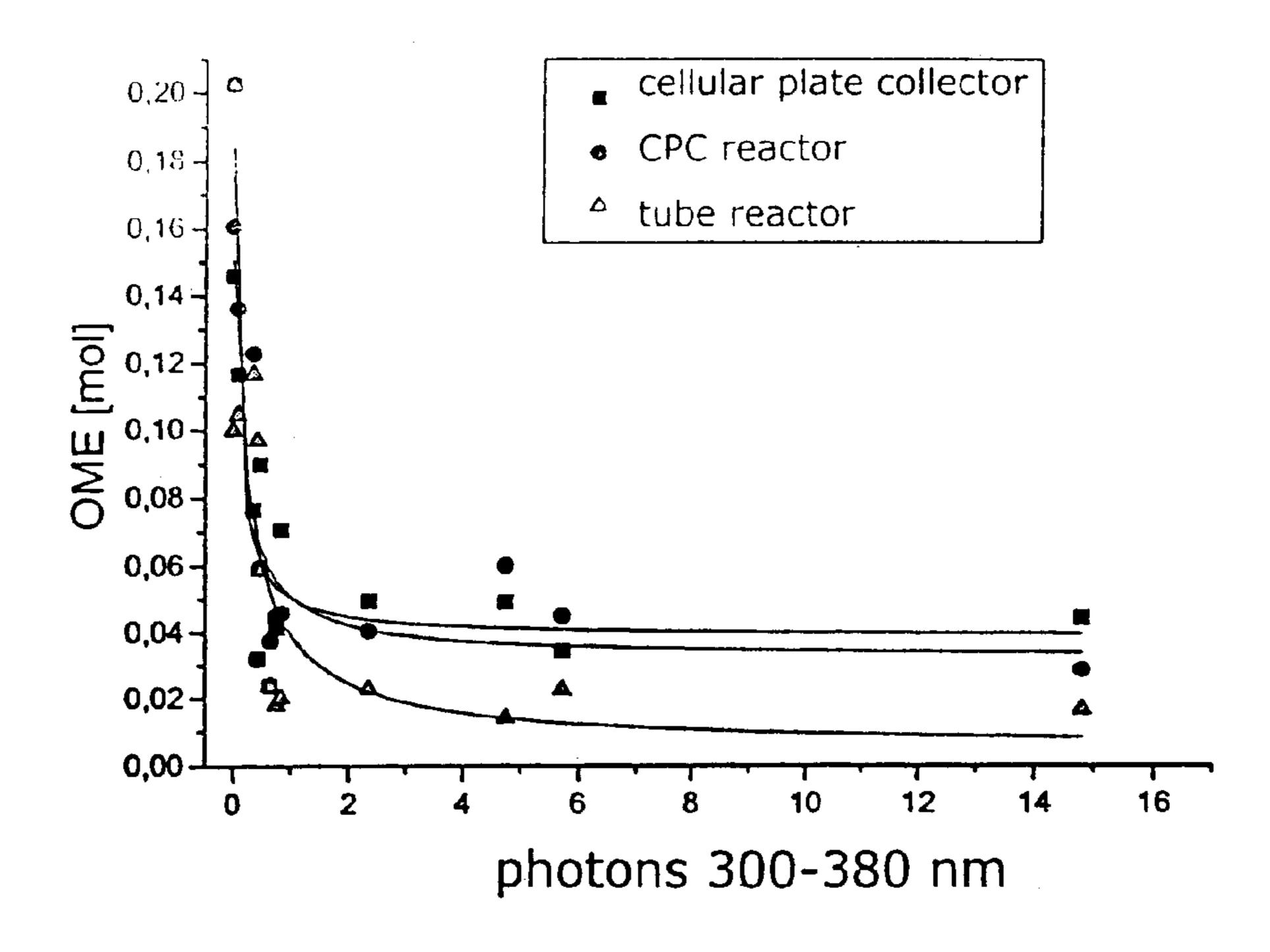
Degradation of OME in water (1000 mg/l) with TiO<sub>2</sub> as a catalyst (200 mg/l)
