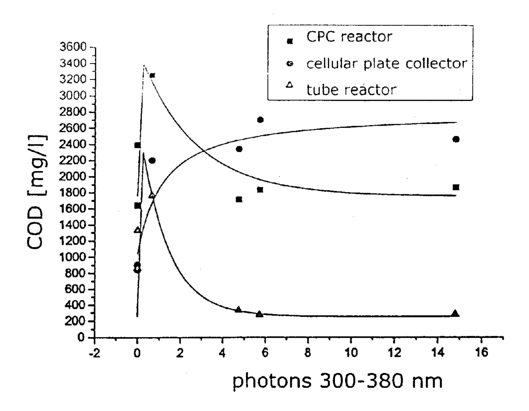
Degradation of OME in water (1000 mg/l) with TiO<sub>2</sub> as a catalyst (200 mg/l)
