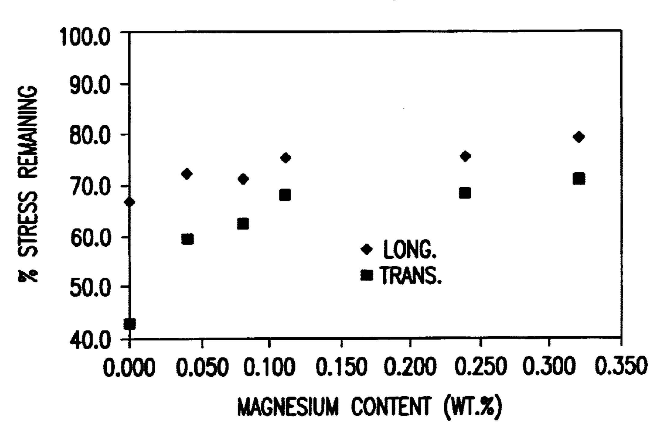
COLD ROLLED 58% RELIEF ANNEALED 275° C/4 HOURS.
