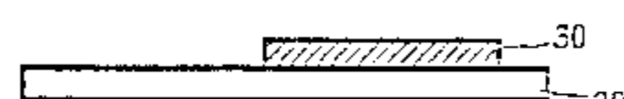
f) ANNEALING AMORPHOUS ITO FILM TO BE CRYSTALLIZED
