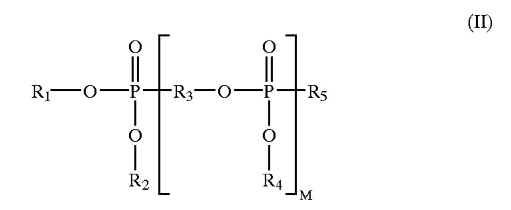
wherein,  $R_1$ ,  $R_2$ ,  $R_4$  and  $R_5$  independently of one another are  $C_6$ – $C_{20}$  aryl or alkyl substituted  $C_6$ – $C_{20}$  aryl,  $R_3$  is alkylene, arylene, or arylene having alkyl group, M is 0 or 1 to 3 when the phosphate ester (D-2) is used alone and M is an average value from 0.1 to 3 when a mixture of phosphate esters (D-2) is used, and
