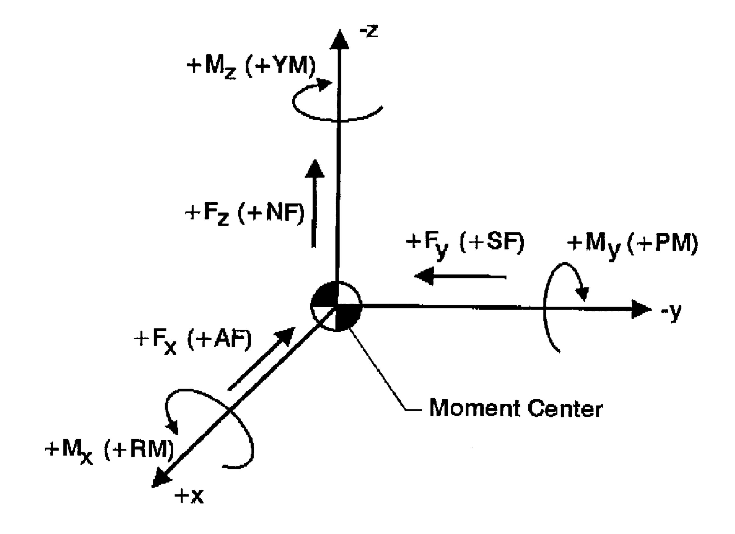
Multi-axis Load Cell Coordinate System
