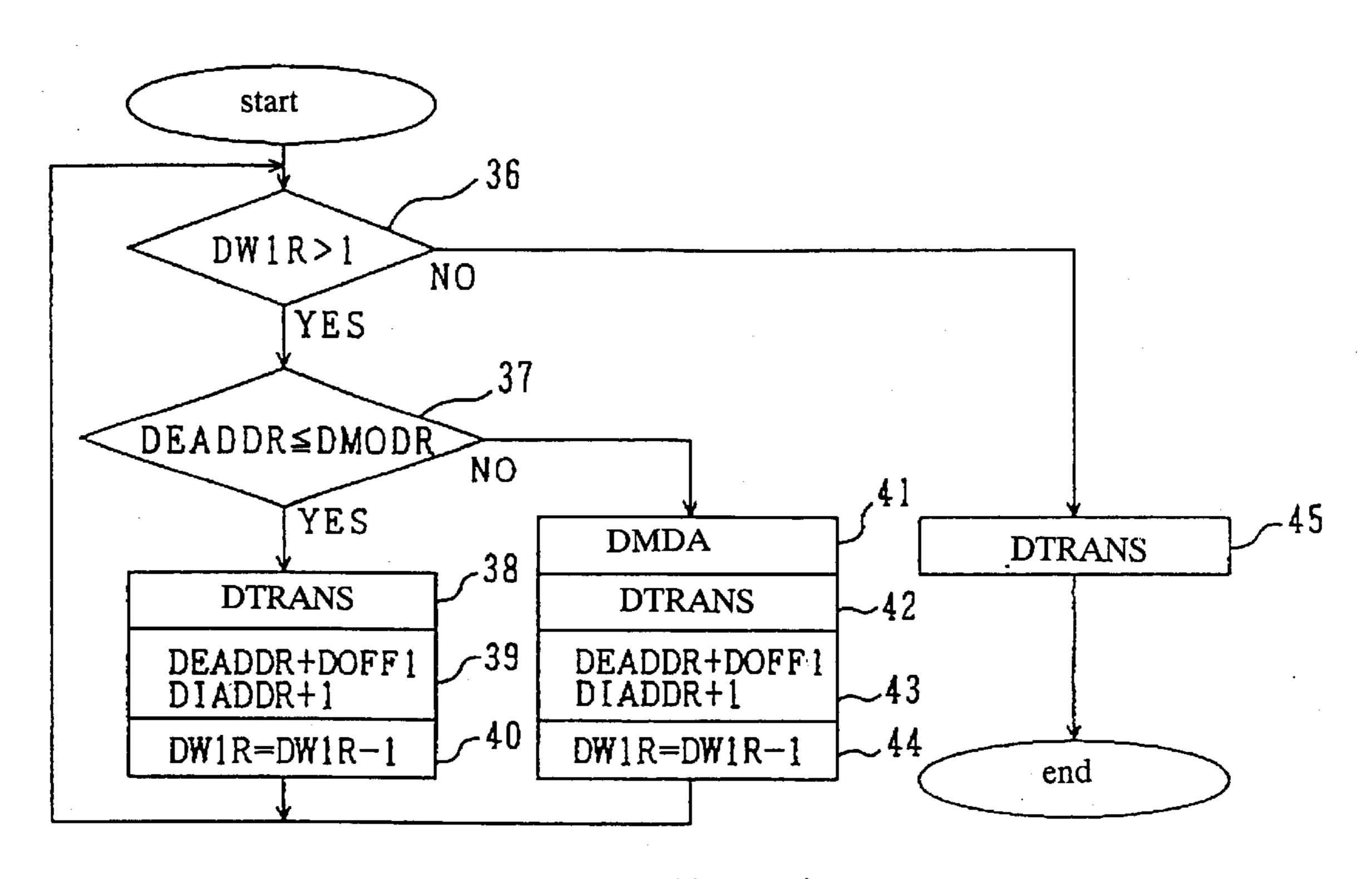
DEADDR: external memory address register DIADDR: internal memory address register
