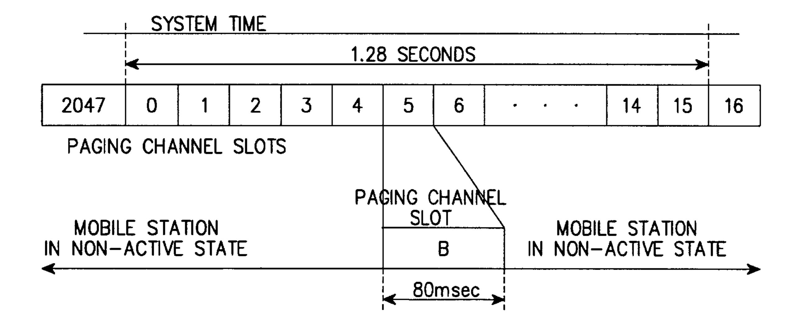
5-MOBILE STATION'S ASSIGNED PAGING CHANNEL SLOT
