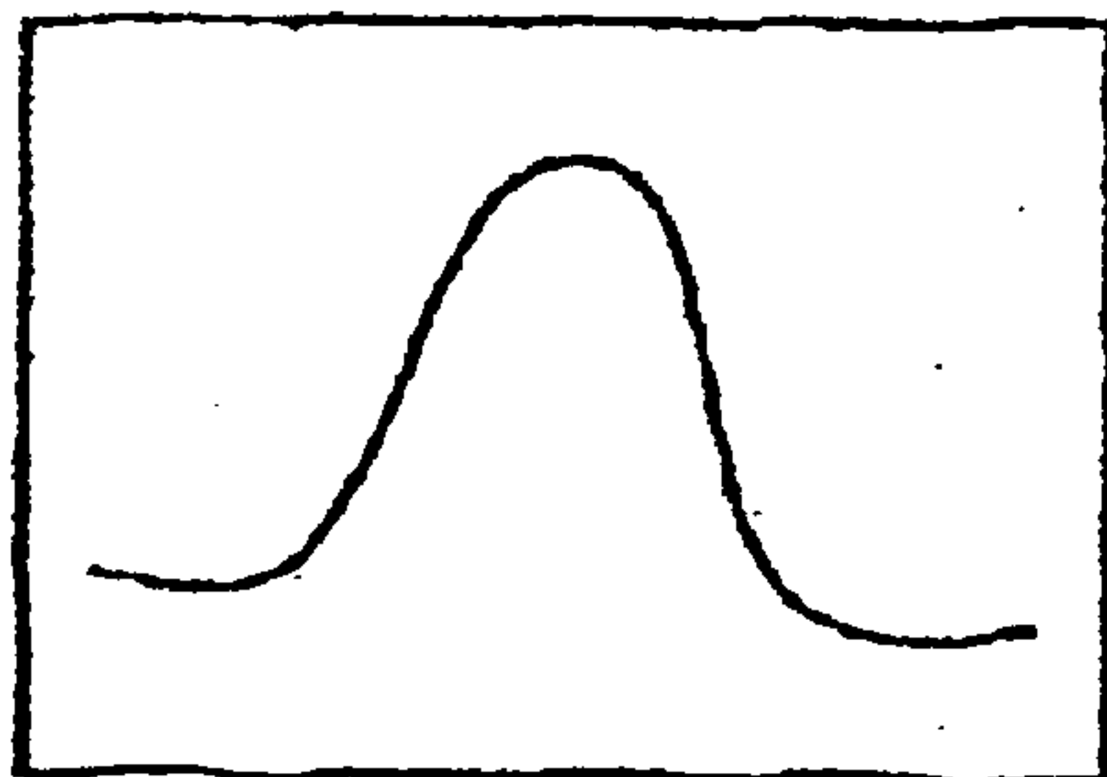
Normal Waveform of Radiation detector
