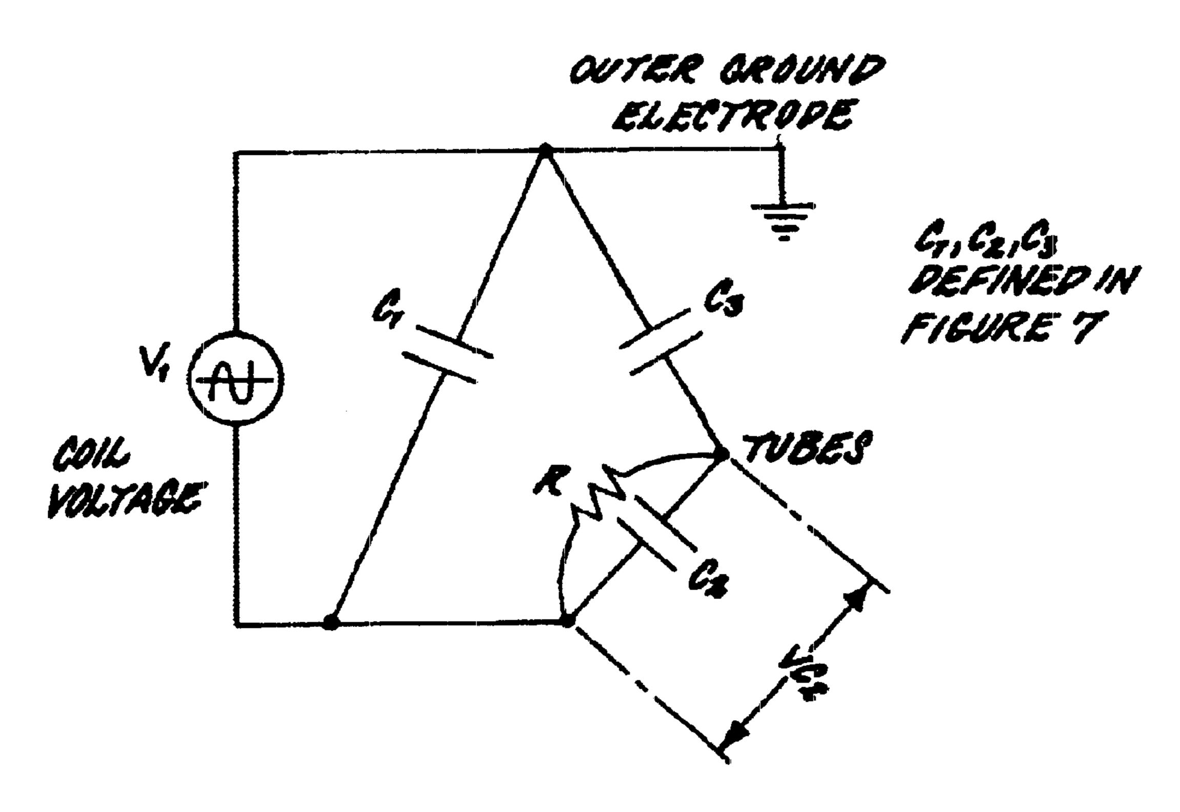
VOLTAGE BETWEEN TUBES AND COPPER = VC2 WITHOUT R  $VC_2 = \frac{\chi C_2}{\chi C_3 + \chi C_2} \cdot V_1$   $\chi$ =CAPACITOR REACTANCE R = VOLTAGE GRADING RESISTOR  $VC_2 = \frac{R}{\chi C_3 + R} \cdot V_1$  (WITH R IN CIRCUIT) AND R>>  $\chi C_2$
