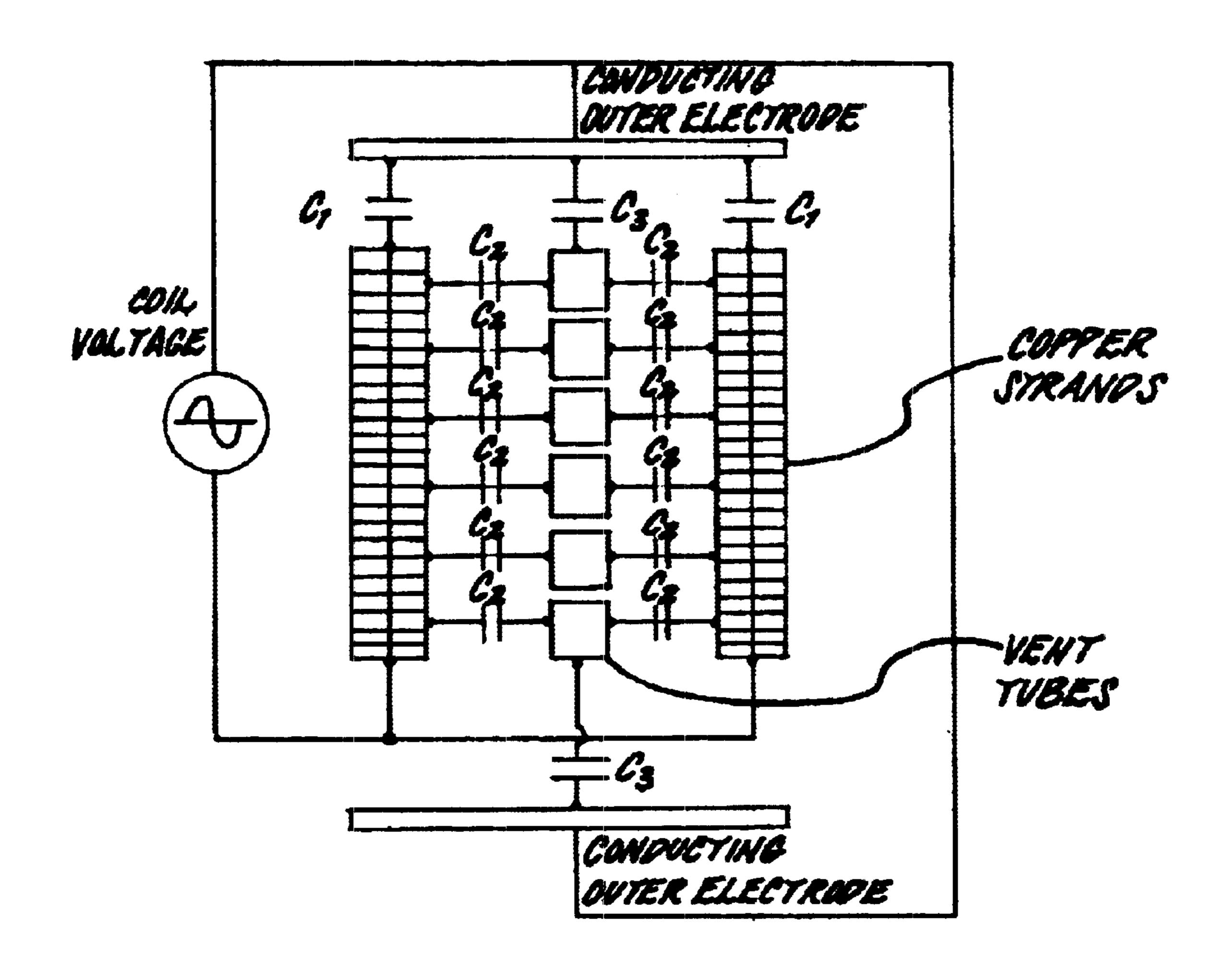
Cy-CAPACITYE COUPLING BETWEEN OUTER ELECTROPE TO COPPER STRANDS
