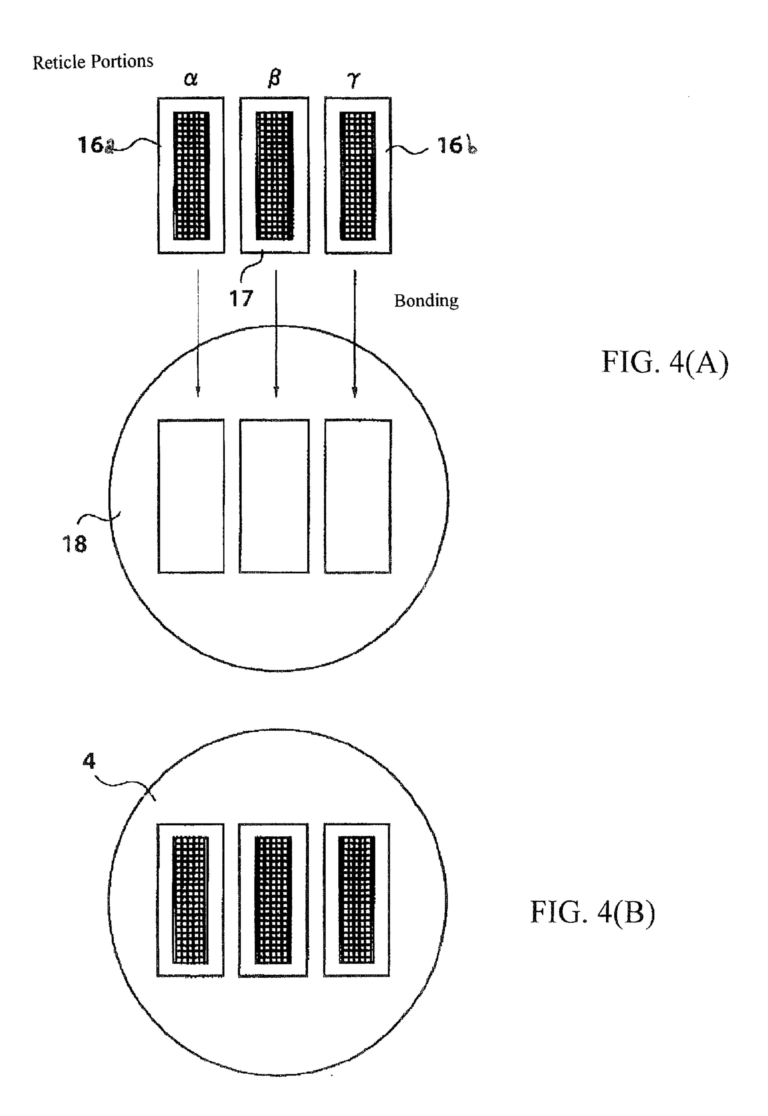
SCATTERING-RETICLE ASSEMBLIES FOR ELECTRON-BEAM MICROLITHOGRAPHY INCLUDING A SCATTERING-STENCIL RETICLE PORTION AND A SCATTERING-MEMBRANE RETICLE PORTION
