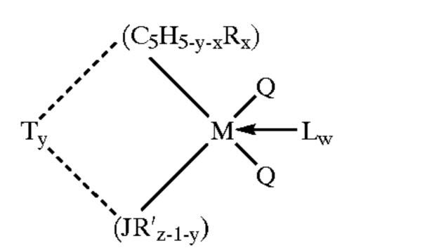
wherein M is Zr, Hf or Ti in its highest formal oxidation state (+4, d<sup>0</sup> complex);
