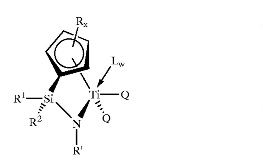
the nature of the R' group may dramatically influence the 50 catalytic properties of the system. For production of ethylene- $\alpha$ -olein copolymers of greatest comonomer content, at a selected ethylene to  $\alpha$ -olefin monomer ratio, R' is preferably a non-aromatic substituent, such as an alkyl or cycloalkyl substituent preferably bearing as primary or 55 secondary carbon atom attached to the nitrogen atom.
