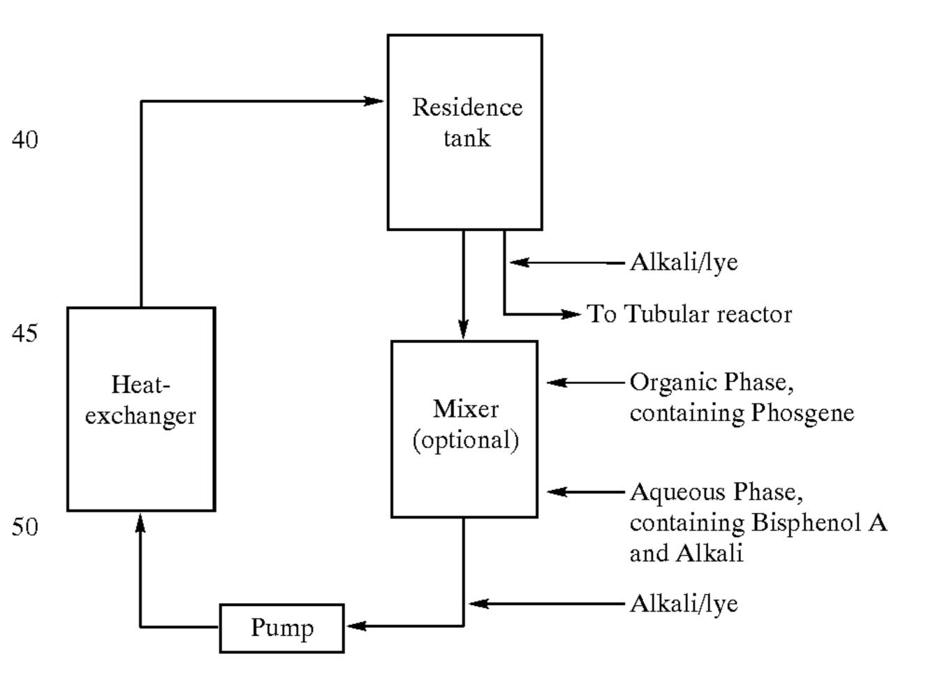
The tubular reactor includes mixing and residence zones and is connected down-stream of the residence tank.
