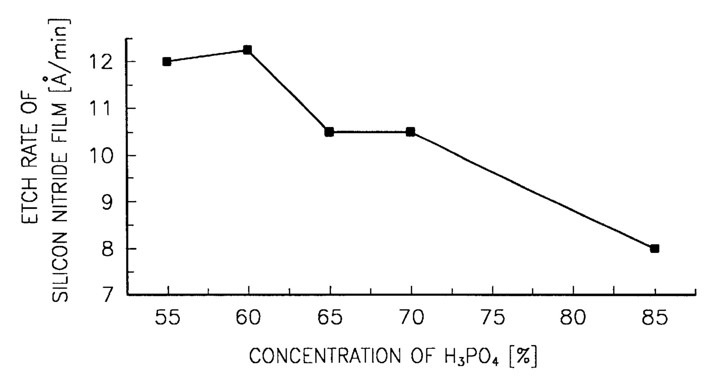
\* ETCH CONDITIONS: 120°C, NO ADDITIVES EXCEPT FOR H<sub>3</sub>PO<sub>4</sub>
