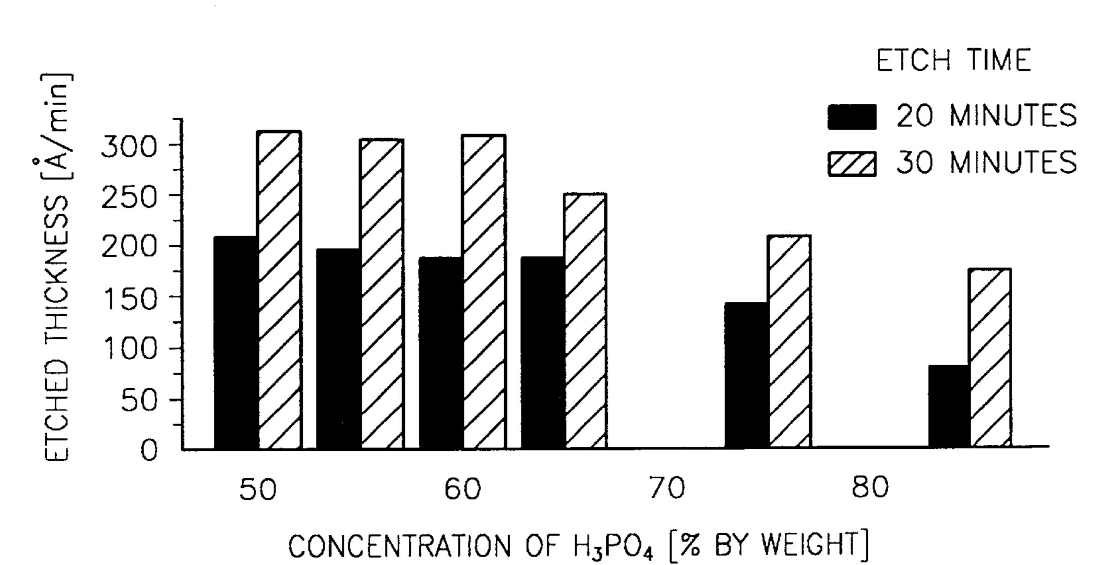
\* ETCH CONDITIONS: 100°C, ADDITION HF OF 0.02% BY WEIGHT
