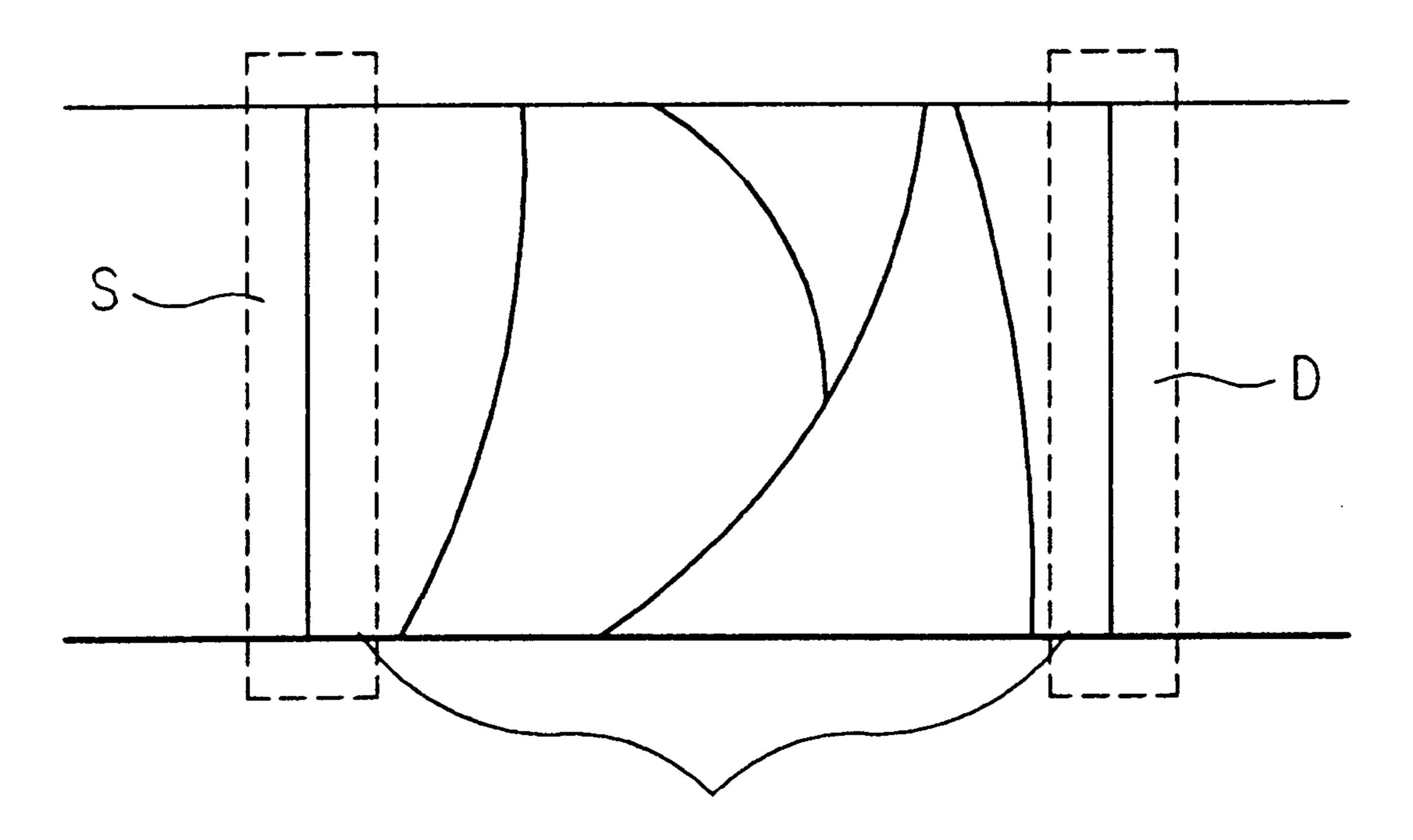
NO GRAIN BOUNDARY WHICH PASSES THROUGH SOURCE "S" AND DRAIN "D"
