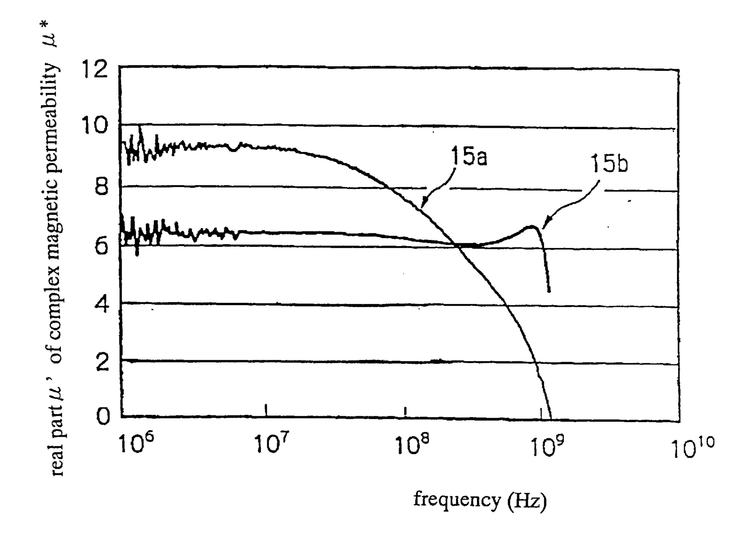
15a: volume ratio of sendust powders to epoxy resin is about 64: 36, averaged particle diameter of sendust powders is about 36  $\mu$  m.
