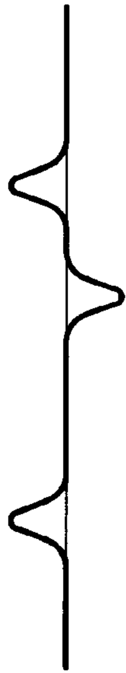
Fig. 1(d) Magnetic flux changes in read head
