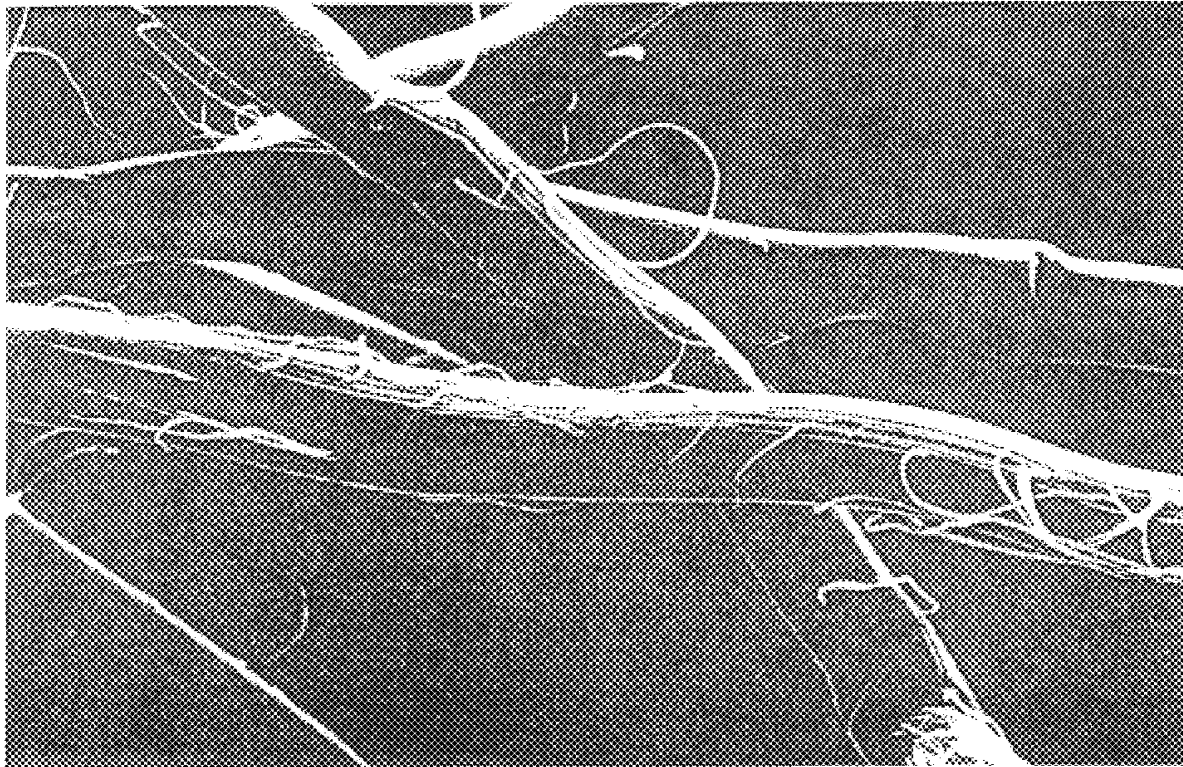
Abraded Commercial Fiber 1 - 1000X
