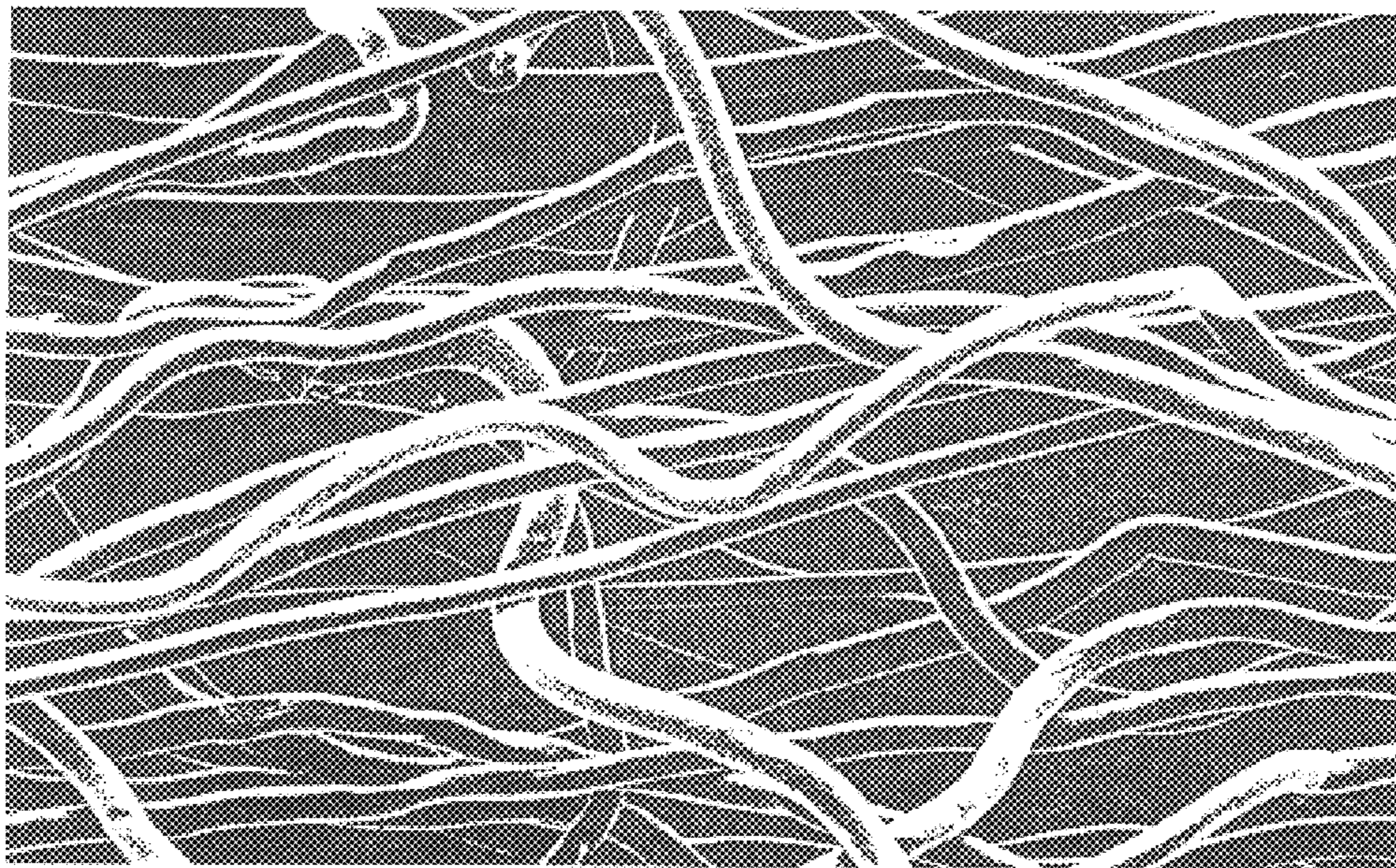
Melt Blown Fiber - 100X
