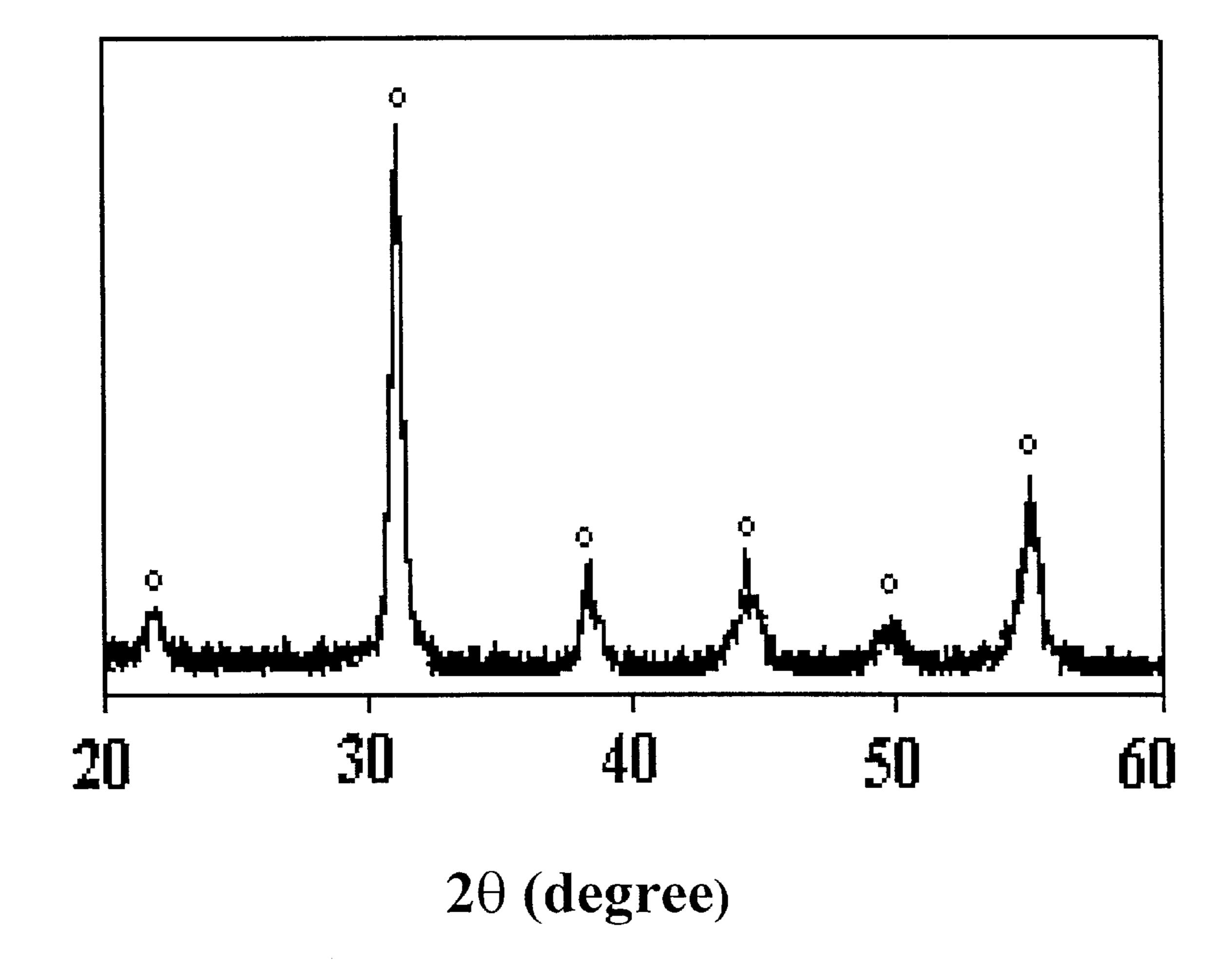
**Figure2** XRD pattern of Pb(Zr<sub>0.52</sub>Ti<sub>0.48</sub>)O<sub>3</sub> sintered at 1050°C for 1 hour
