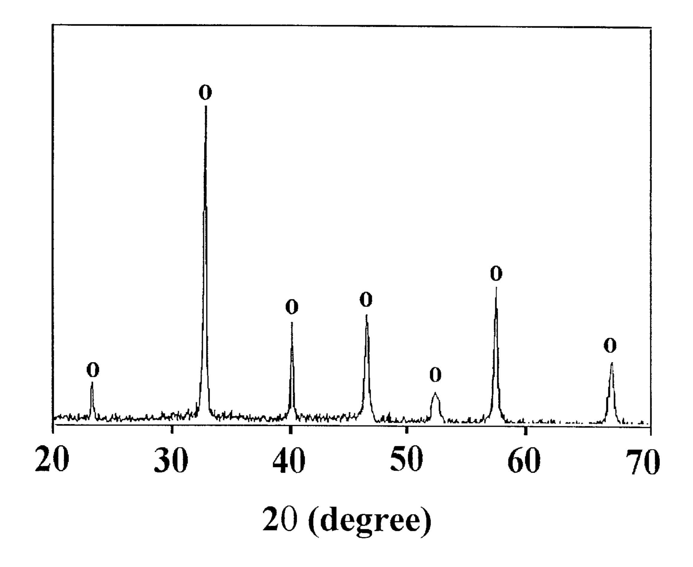
Figure3 XRD pattern of Br<sub>0.65</sub>Sr<sub>0.35</sub>TiO<sub>3</sub> sintered at 1200°C for 1 hour
