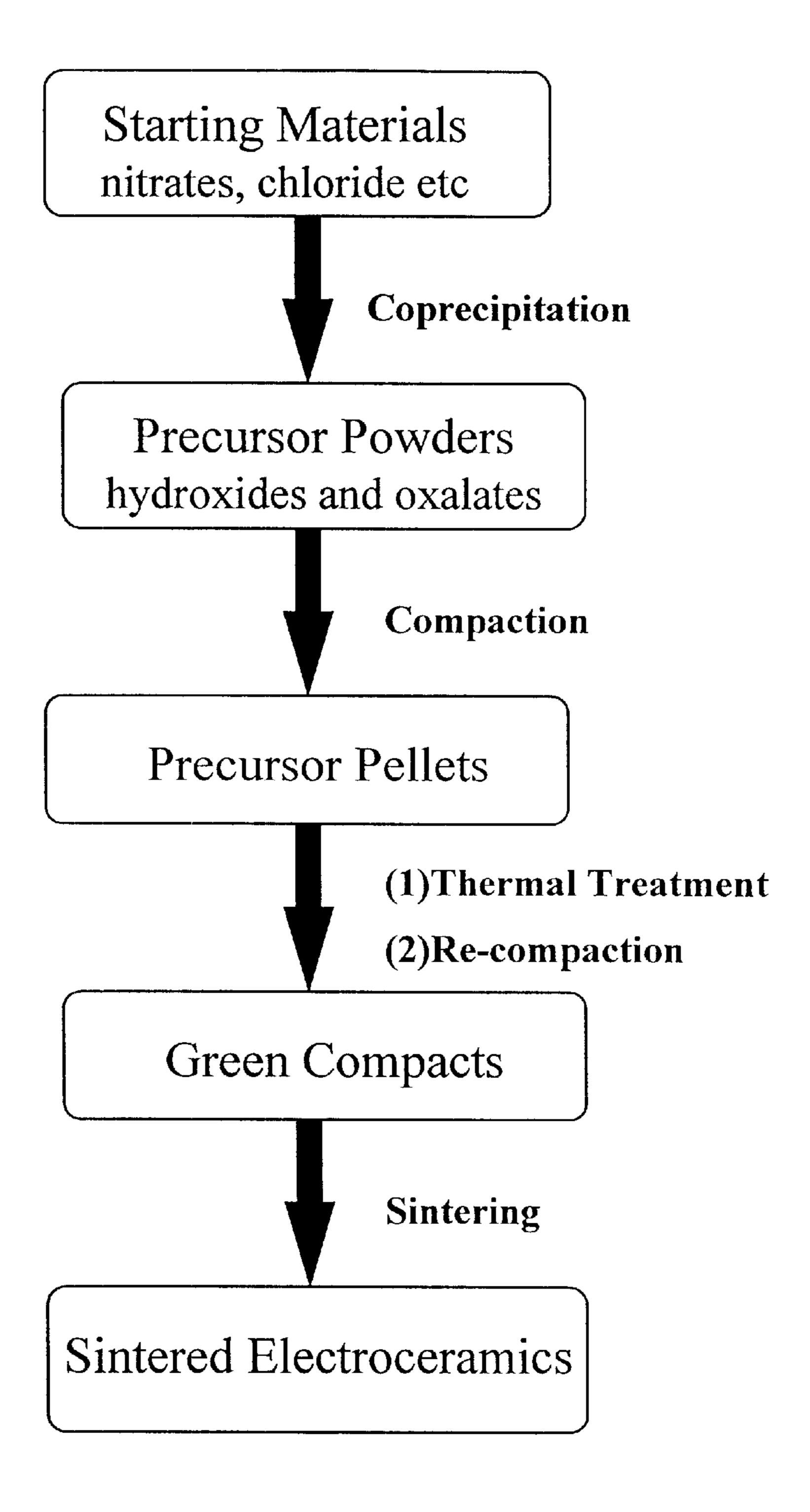
Figure 1 Flow diagram showing the various steps involved in the direct processing technique
