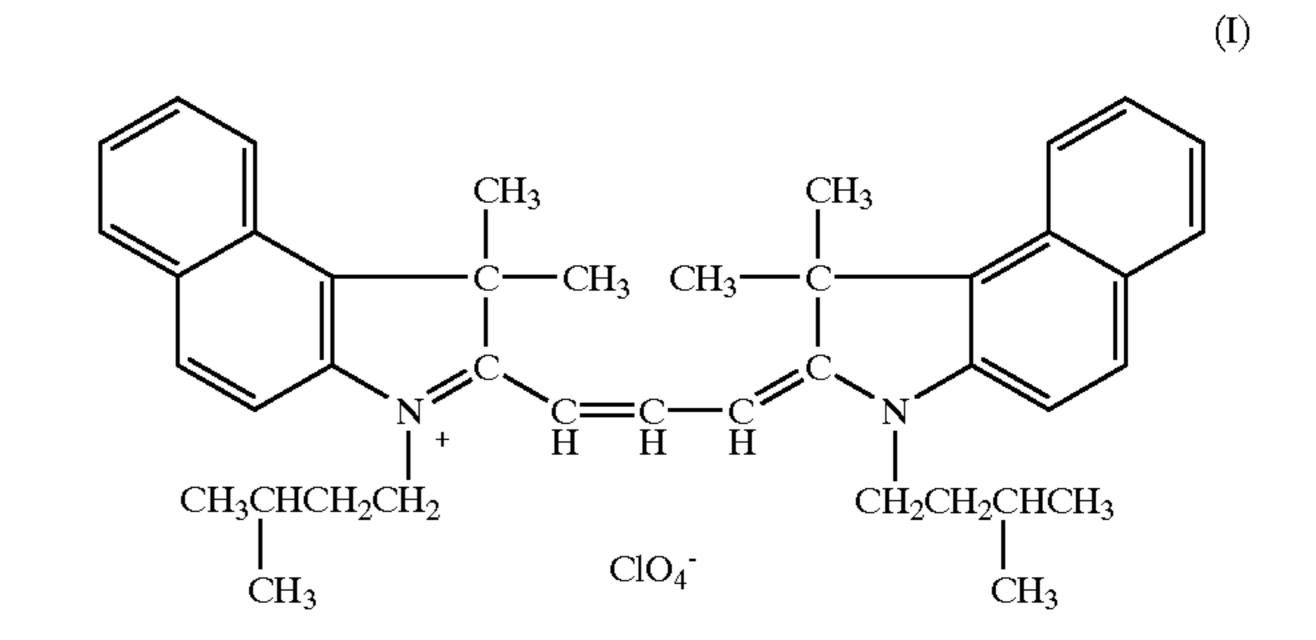
The organic EL device includes a blue color filter made with cyanine dye having the structural formula (I), a glass substrate, an organic protection layer, an inorganic oxide layer, and an organic light-emitting layer including an anode, a hole injection layer, a hole transport layer, a light emitting layer, an electron injection layer and a cathode.
