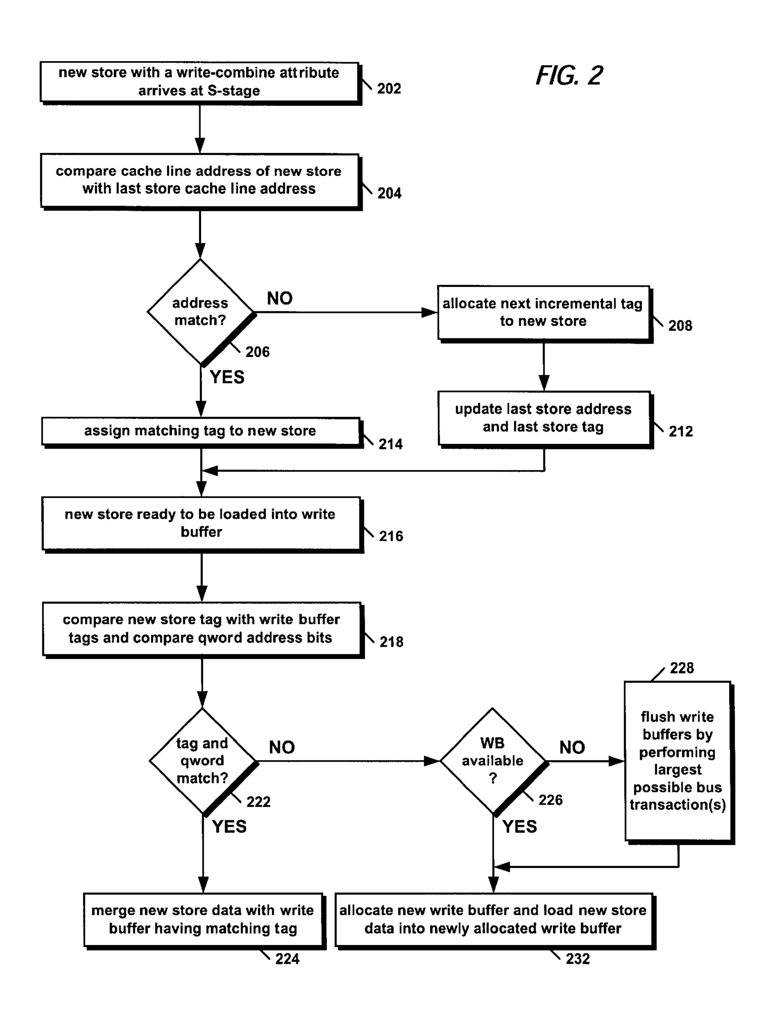
Write-Combining Apparatus Operation
