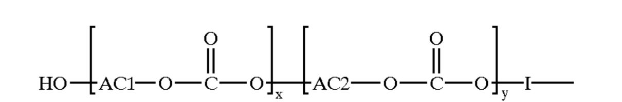
where AC1, AC2, x and y are those defined herein. The photoresist composition has excellent transparency in deep ultraviolet region, etching resistance and heat resistance, and can form a good pattern without a developing step. Accordingly, the photoresist composition can be applied to a high density minute pattern below  $0.15 \mu m$  (e.g., for fabrication of DRAM over 1G), and efficiently employed for the lithography process using ArF, KrF, VUV, EUV, E-beam and X-ray.
