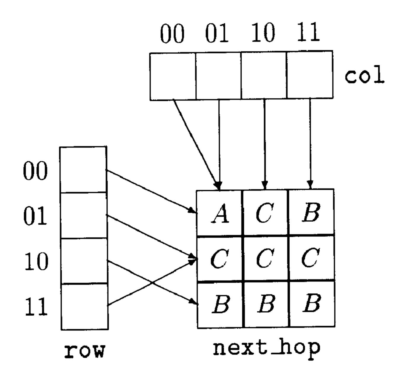
Figure 1: The overall IP address lookup data structures
