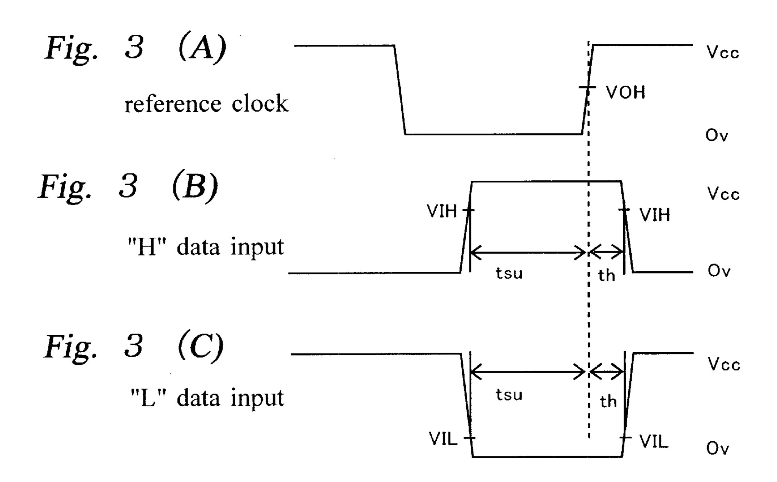
(setup times)tsu ≤product specification tsu (hold times)th≤prouct specification th
