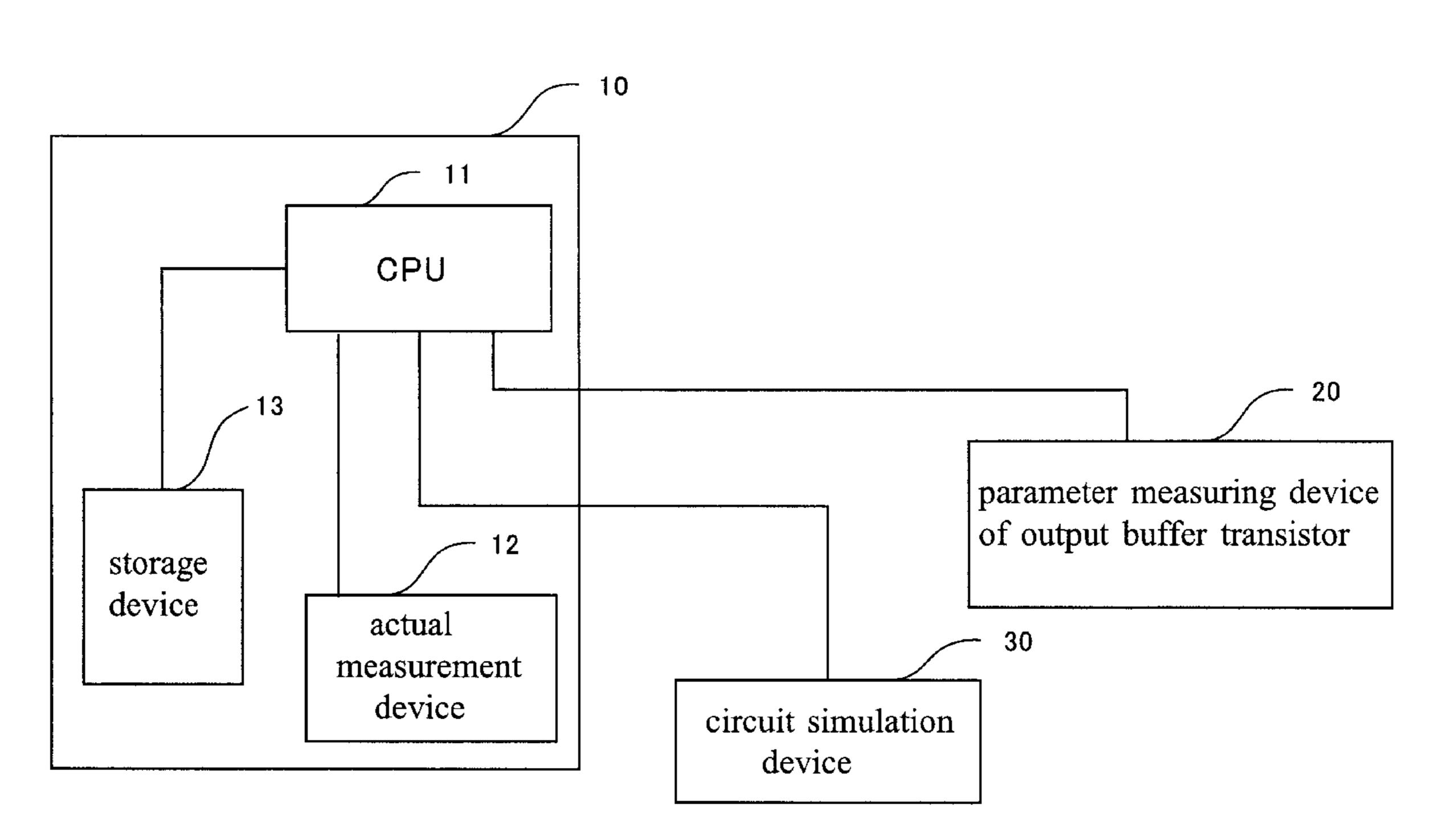
parameter measuring devi of output buffer transistor of output be circuit simulation device measurement 12 device actual storage device
